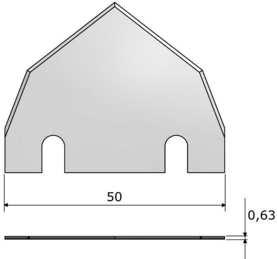
Double arrow shaped blade. Superb performance in materials like Kappa and foamed core board. Works with fluted core boards and triple wall corrugated. Made from a special Tungsten Carbide alloy to extend lifetime
