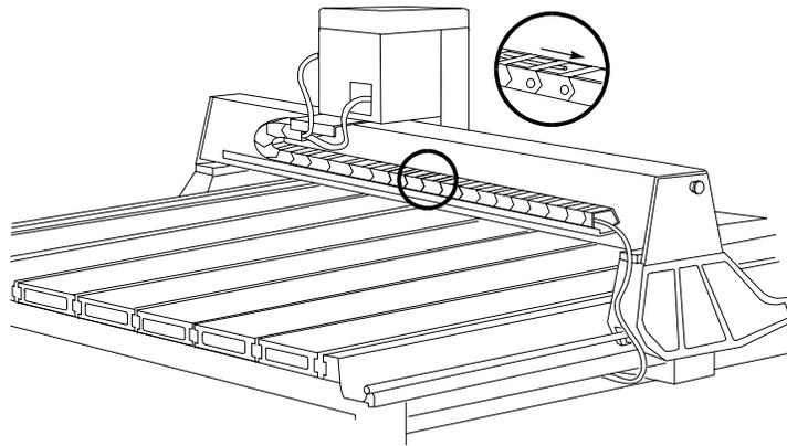
6. Pull the hoses out of the cable carrier, then feed them back into the carrier through the same slot. Pulling them out first makes feeding them through the remaining section of the carrier easier.
