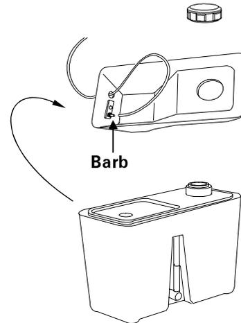
3. Feed the black hose with the red stripe (coolant hose) through the yellow cap supplied in the kit as shown in the illustration.
