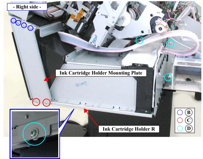
Figure 4-133. Removing the Ink Cartridge Holder R
