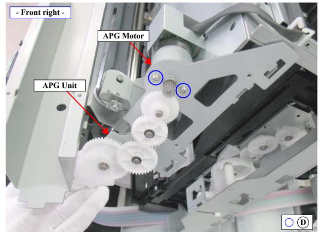
Figure 4-74. Removing the APG Motor
