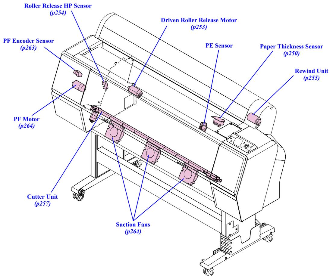
Figure 4-8. Paper Feed Mechanism
