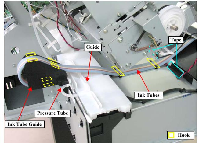
Figure 4-134. Releasing the Waste Ink Tube and Pressure Tube (before released)
