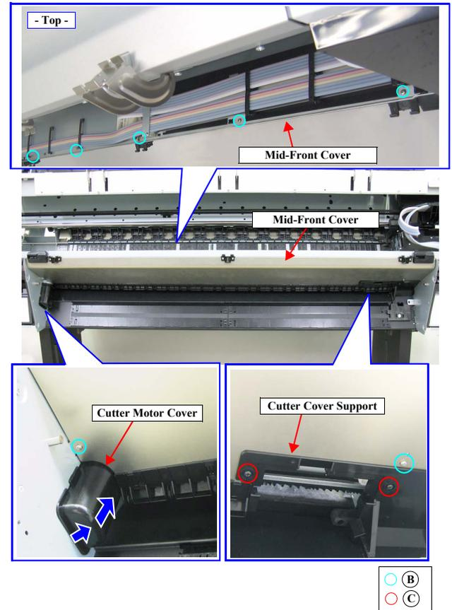
Figure 4-95. Removing the Mid-Front Cover
