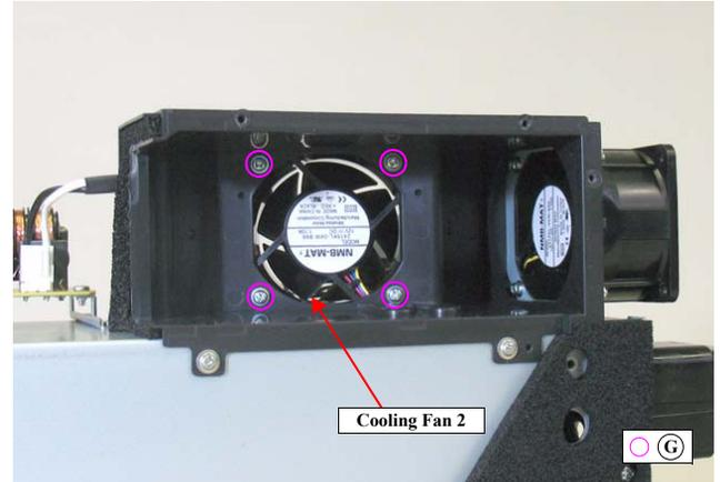
Figure 4-223. Removing the Cooling Fan 2 (2)
