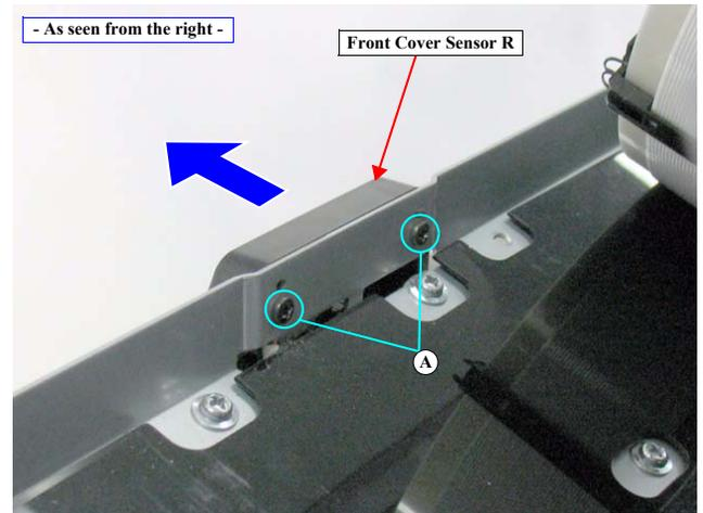
Figure 4-38. Removing the Front Cover Sensor R
