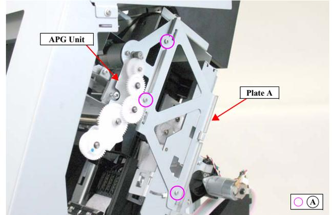
Figure 4-71. Removing the Plate A
