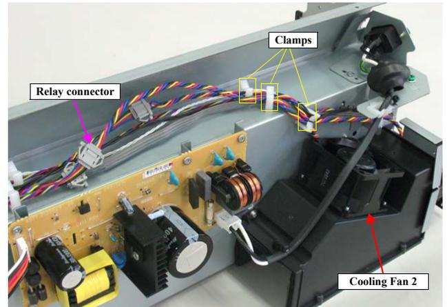
Figure 4-222. Removing the Cooling Fan 2 (1)
