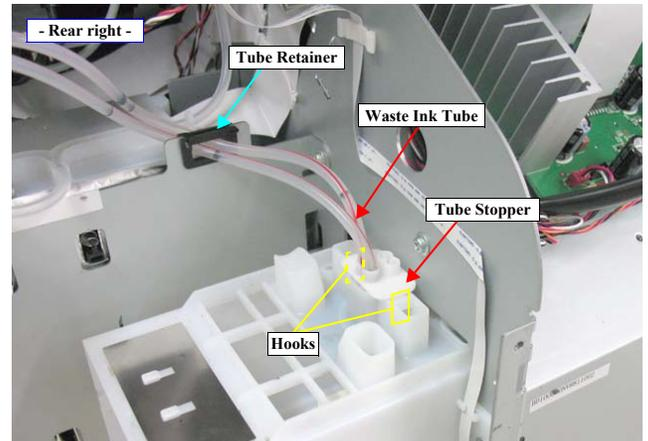
Figure 4-107. Disconnecting the Waste Ink Tube
