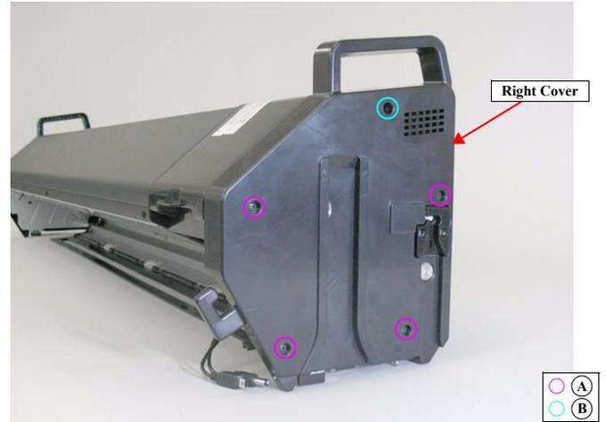
Figure 4-197. Removing the Right Cover
