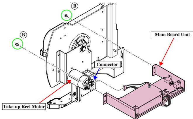
Figure 4-184. Removing the Main Board Unit
