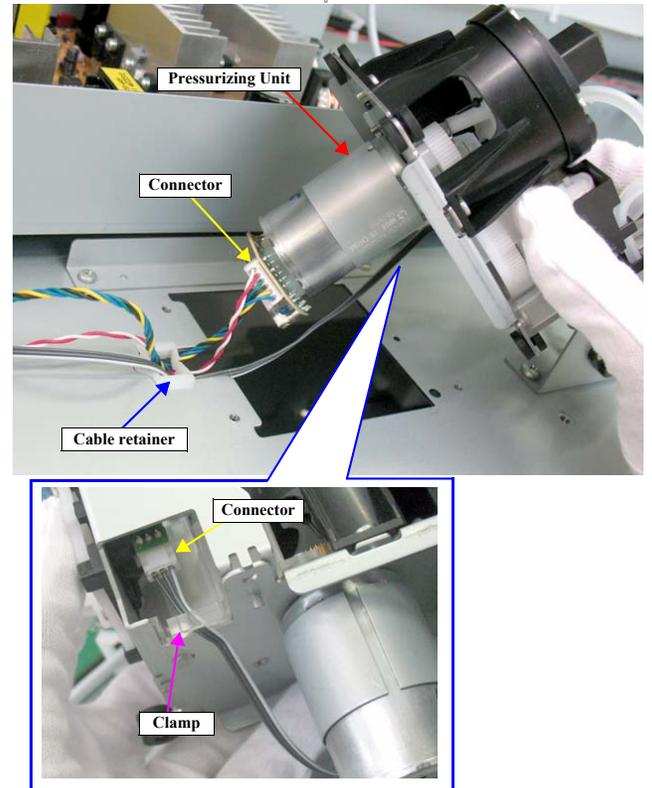
Figure 4-124. Removing the Pressurizing Unit
