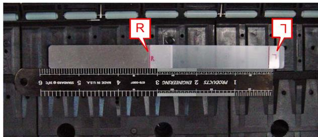
Figure 5-18. Position of the Adjustment jig
