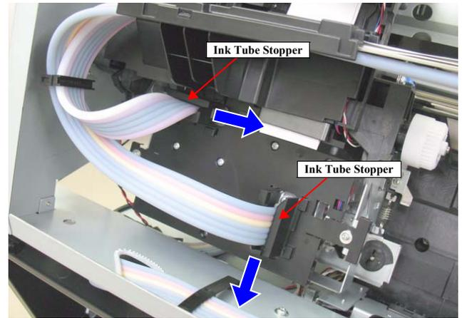
Figure 4-158. Removing the Ink Tube Stopper
