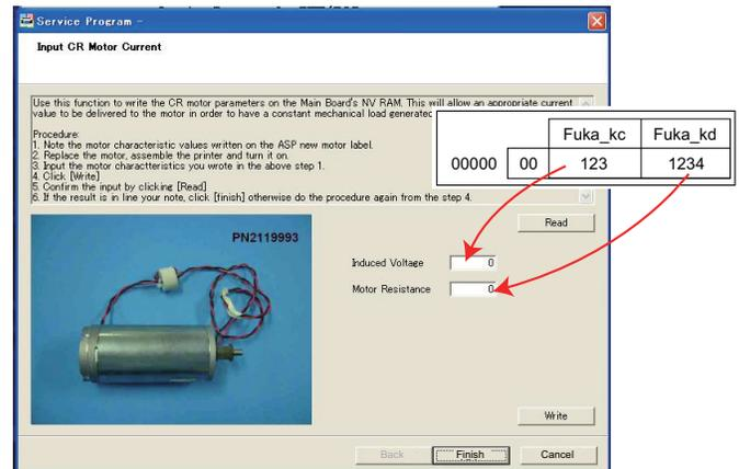
Figure 5-77. [Input CR Motor Current] Screen
