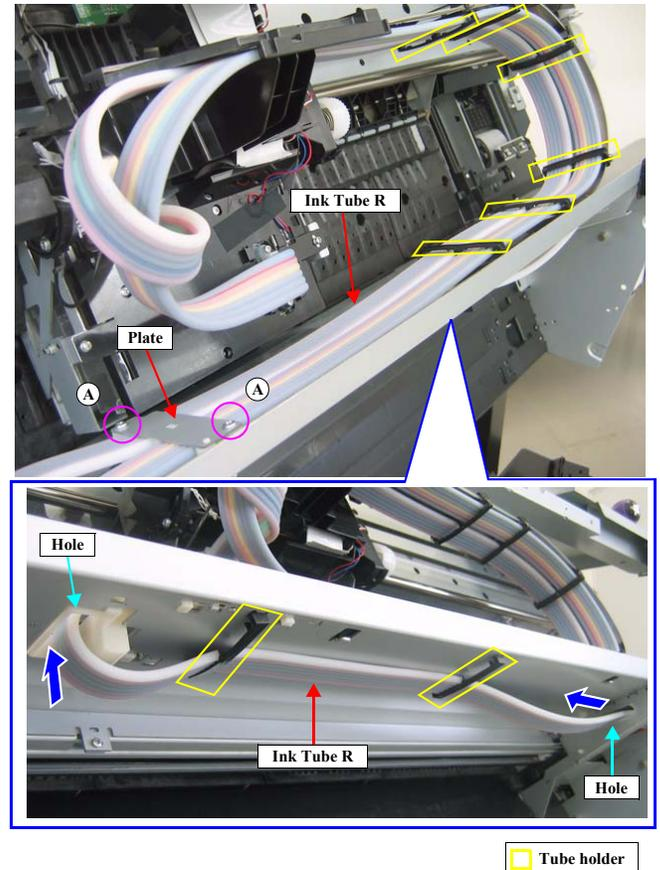
Figure 4-163. Releasing the Ink Tube R
