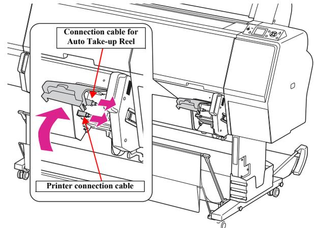
Figure 4-193. Disconnecting the cables (1)
