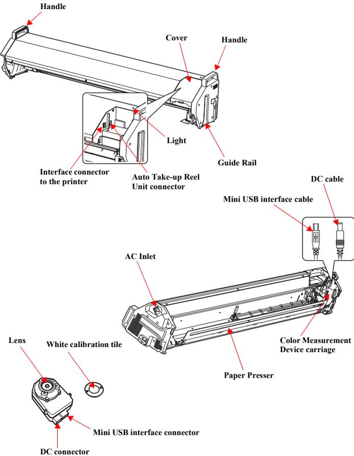
Figure 1-8. Part Names (SpectroProofer)
