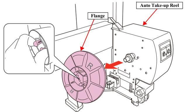
Figure 4-182. Removing the Flange
