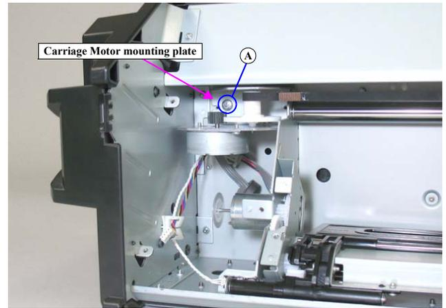
Figure 4-224. Removing the Carriage Motor mounting plate
