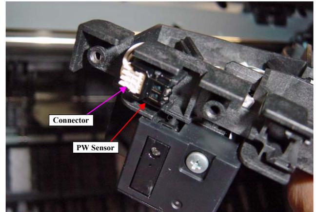
Figure 4-86. Removing the PW Sensor
