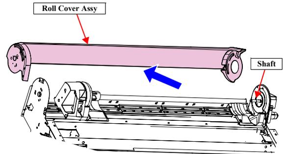
Figure 4-33. Removing the Roll Cover Assy
