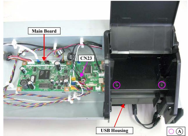
Figure 4-212. Removing the USB Housing
