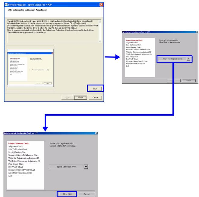
Figure 5-40. Colorimetric Calibration ID Startup Screen
