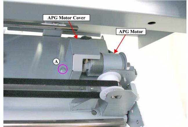
Figure 4-69. Removing the APG Motor (1)
