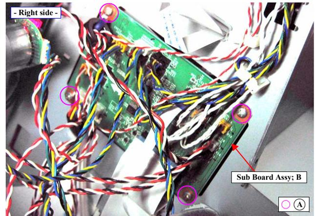
Figure 4-55. Removing the Sub Board Assy; B
