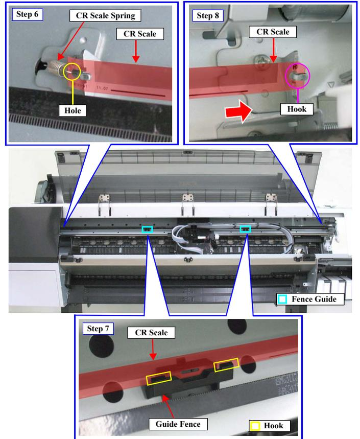
Figure 4-58. Removing the CR Scale
