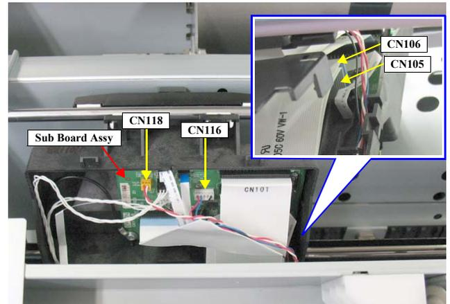
Figure 4-155. Disconnecting the connectors
