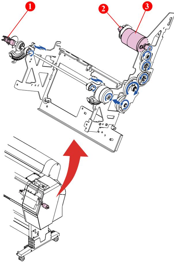
Figure 2-4. Paper Feed Mechanism
