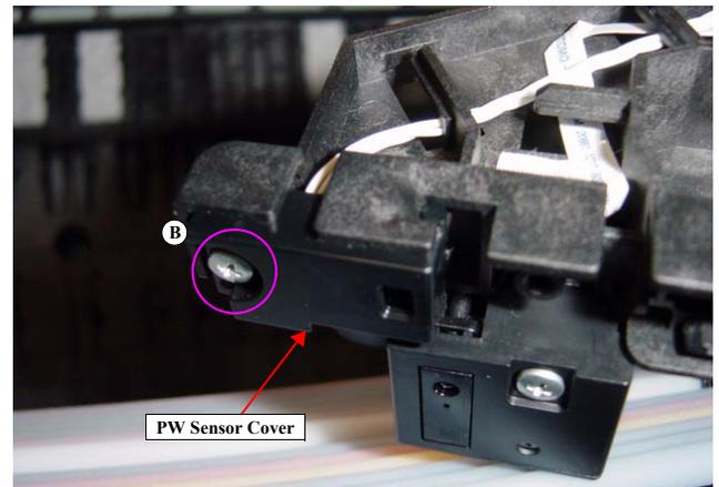
Figure 4-85. Removing the PW Sensor Cover
