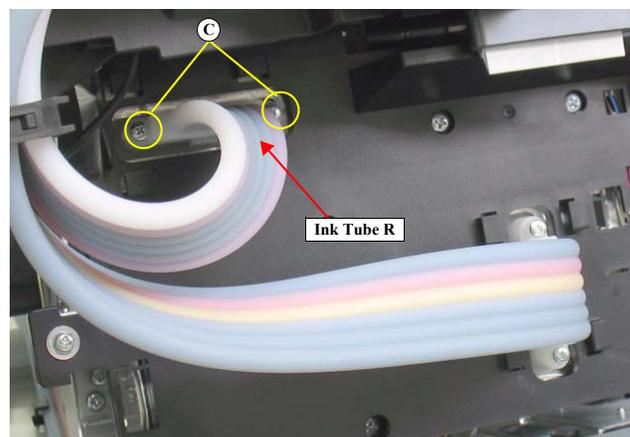
Figure 4-166. Removing the Ink Tube R
