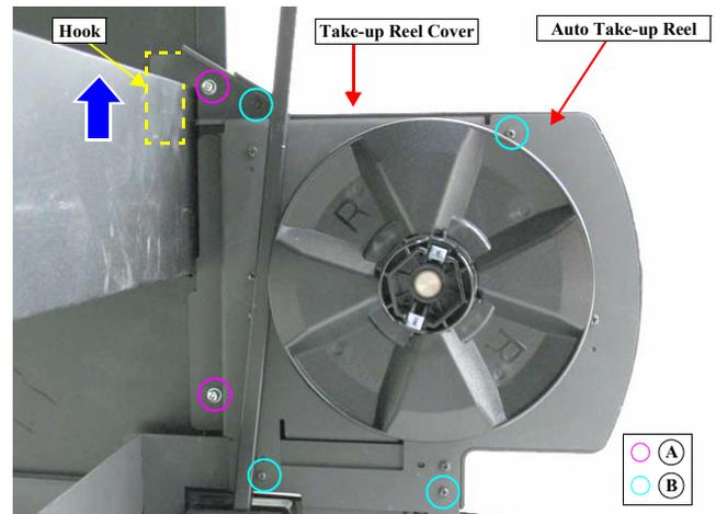
Figure 4-170. Removing the Auto Take-up Reel
