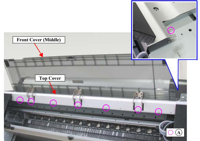
Figure 4-26. Removing the Top Cover (1)
