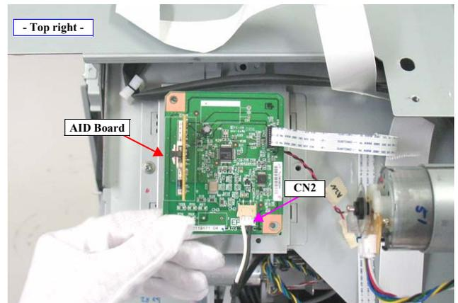
Figure 4-110. Disconnecting the connector on the AID Board.
