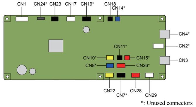
Figure 4-190. Connector location
