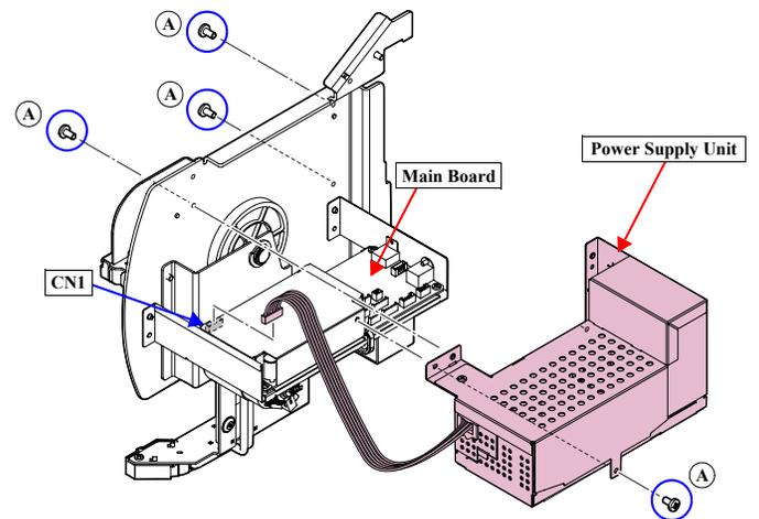
Figure 4-183. Removing the Power Supply Unit
