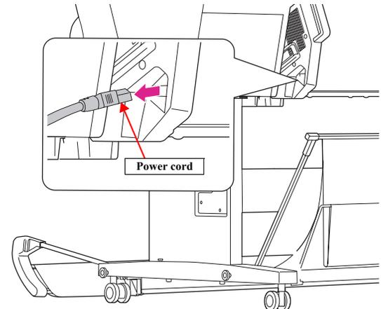
Figure 4-192. Detaching the power cord
