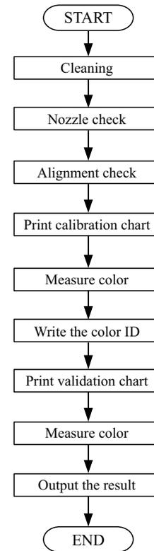
Figure 5-39. Adjustment Workflow
