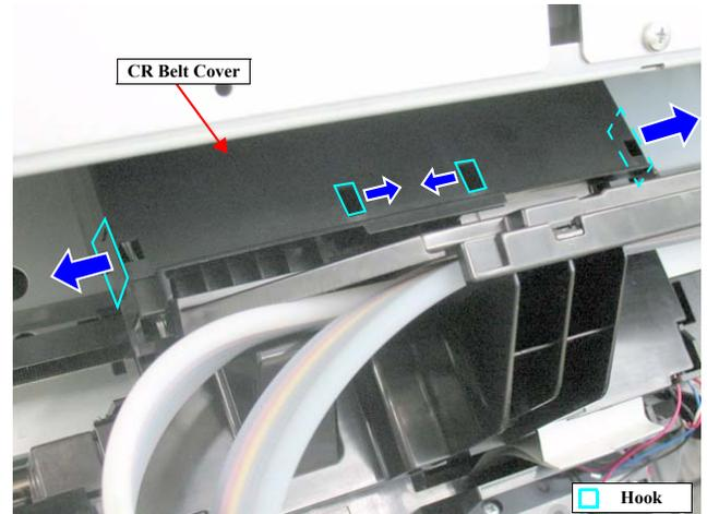
Figure 4-51. Removing the CR Belt Cover
