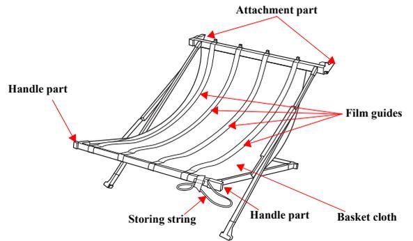
Figure 1-6. Part Names (Basket for Epson Special Film)
