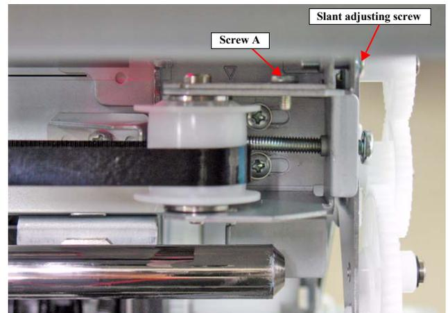
Figure 5-13. Slant Adjusting Screw
