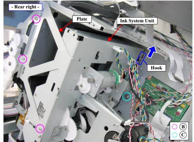
Figure 4-111. Removing the Ink System Unit
