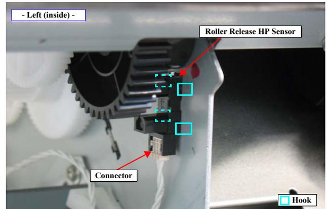
Figure 4-89. Removing the Roller Release HP Sensor
