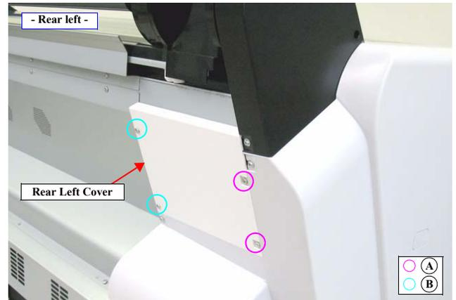
Figure 4-34. Removing the Rear Left Cover
