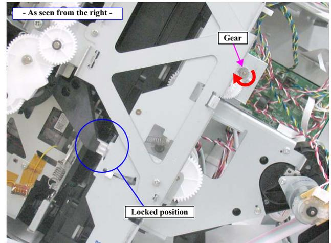
Figure 4-12. Unlocking the Carriage Unit
