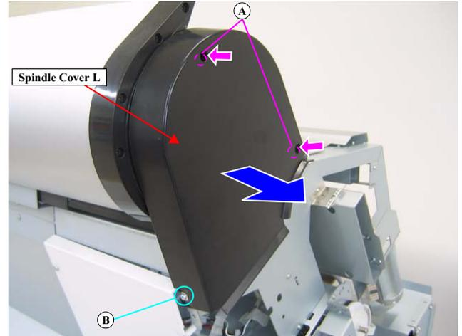
Figure 4-30. Removing the Spindle Cover L
