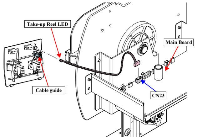
Figure 4-175. Removing the Take-up Reel LED
