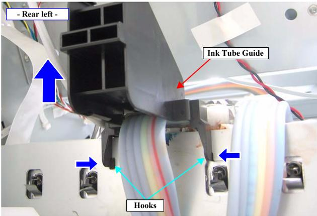
Figure 4-136. Removing the Ink Tube Guide
