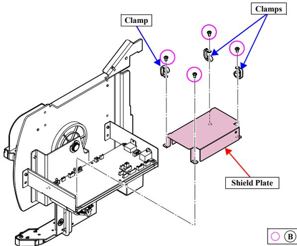
Figure 4-189. Removing the Shield Plate
