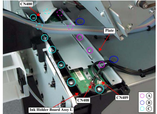
Figure 4-143. Removing the Ink Holder Board Assy L
