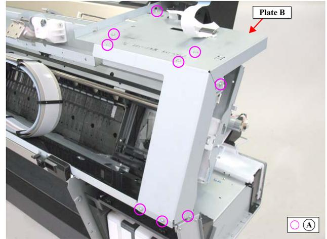
Figure 4-79. Removing the Plate B
