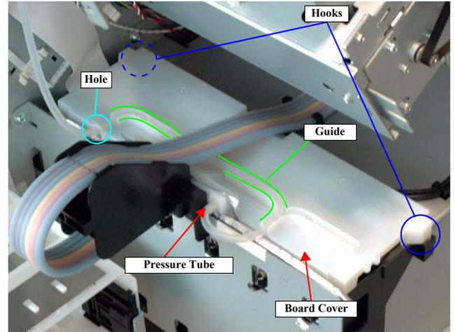
Figure 4-142. Removing the Board Cover
