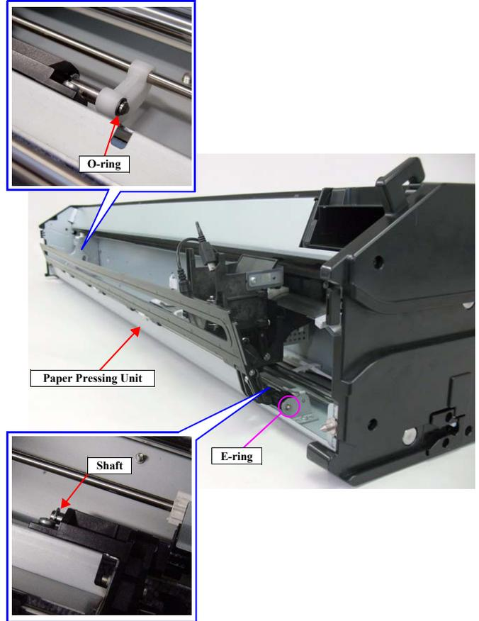
Figure 4-231. Removing the Paper Pressing Unit
