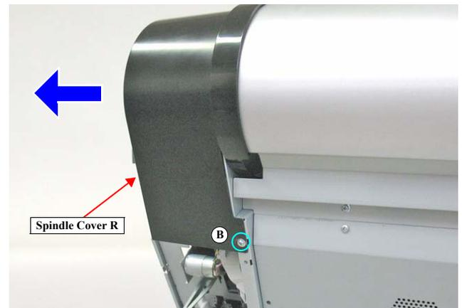
Figure 4-29. Removing the Spindle Cover R
