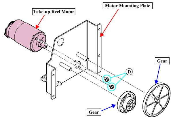
Figure 4-186. Removing the Take-up Reel Motor
