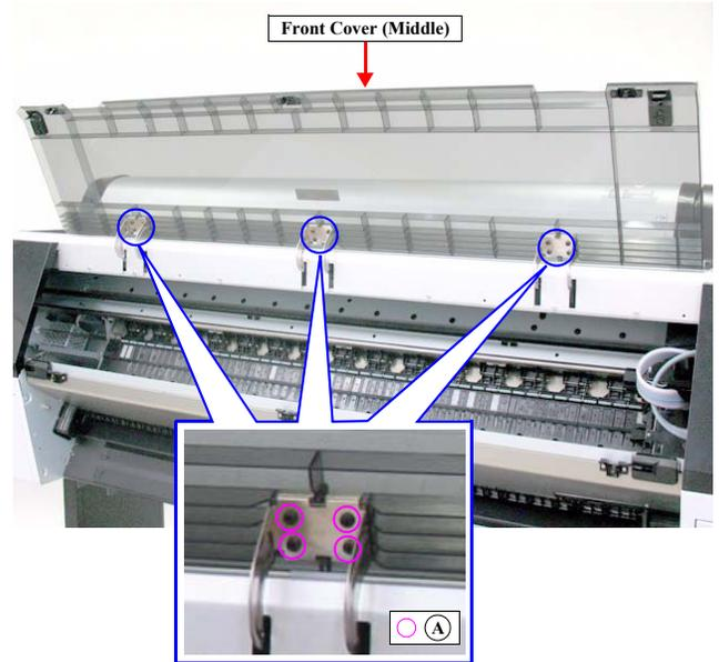
Figure 4-25. Removing the Front Cover (Middle)
