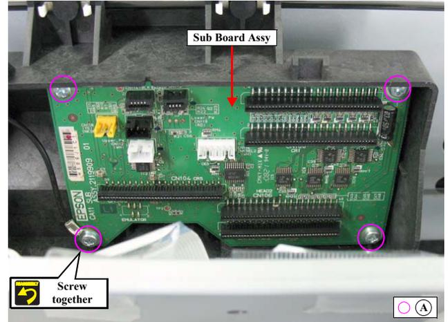
Figure 4-53. Removing the Sub Board Assy
