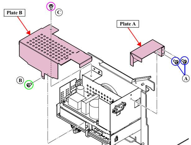
Figure 4-180. Removing the Plate A/B
