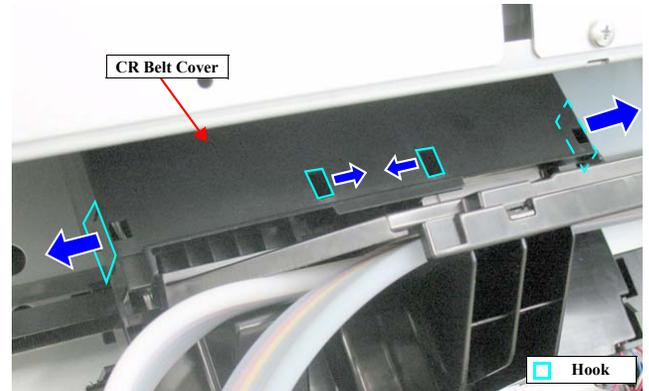
Figure 4-154. Removing the CR Belt Cover
