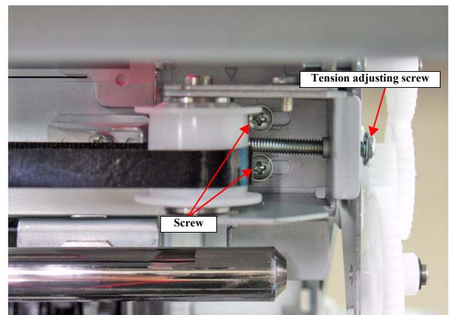
Figure 5-16. Tension Adjusting Screw
