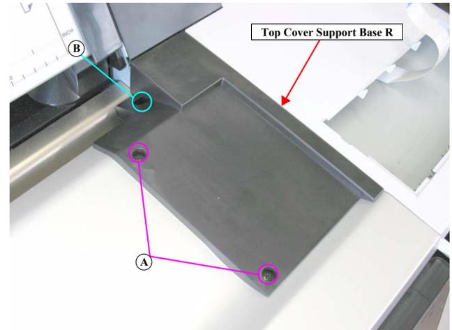
Figure 4-21. Removing the Top Cover Support Base R
