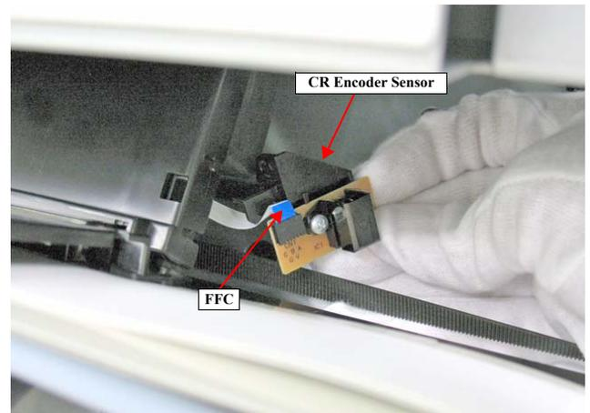
Figure 4-60. Disconnecting the FFC
