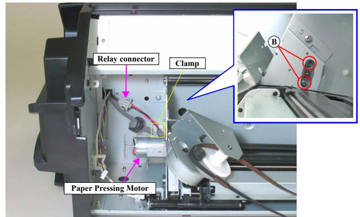
Figure 4-225. Removing the Paper Pressing motor
