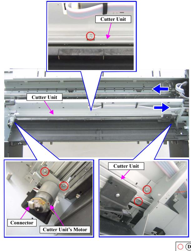
Figure 4-98. Removing the Cutter Unit
