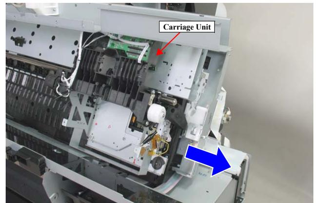
Figure 4-81. Remove the Carriage Unit
