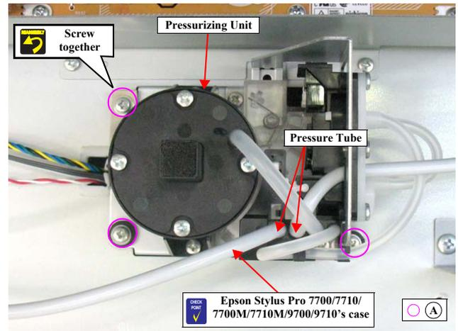
Figure 4-123. Removing the screws securing the Pressurizing Unit
