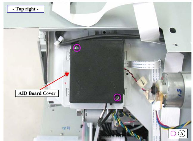
Figure 4-147. Removing the AID Board Cover
