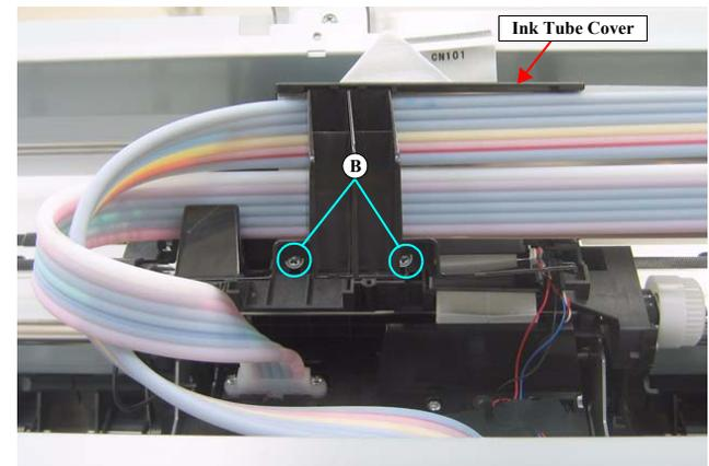
Figure 4-165. Removing the Ink Tube Cover
