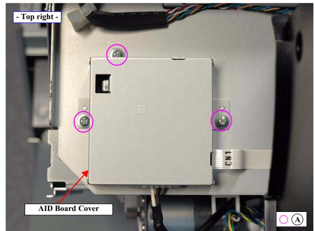
Figure 4-149. Removing the AID Board Cover
