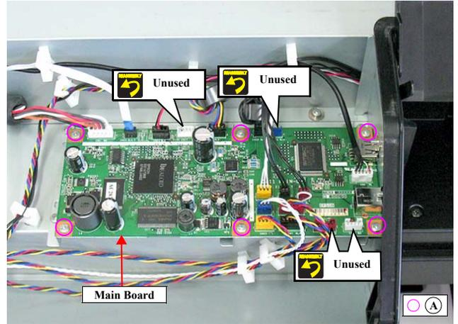
Figure 4-203. Removing the Main Board (1)
