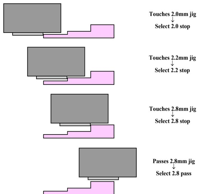
Figure 5-22. Contact point and the set values
