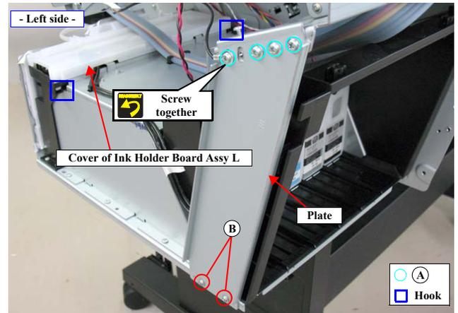
Figure 4-45. Removing the Cartridge Cover Sensor L
