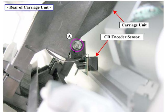
Figure 4-59. Removing the CR Encoder Sensor
