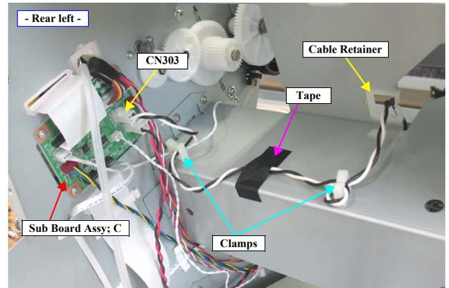
Figure 4-104. Releasing the harness
