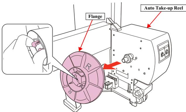
Figure 4-173. Removing the Flange
