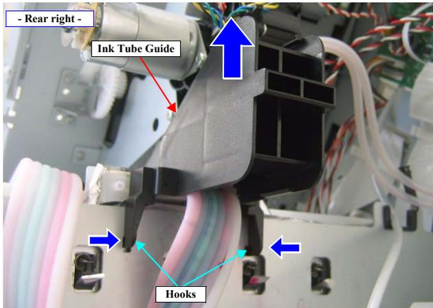
Figure 4-128. Removing the Ink Tube Guide
