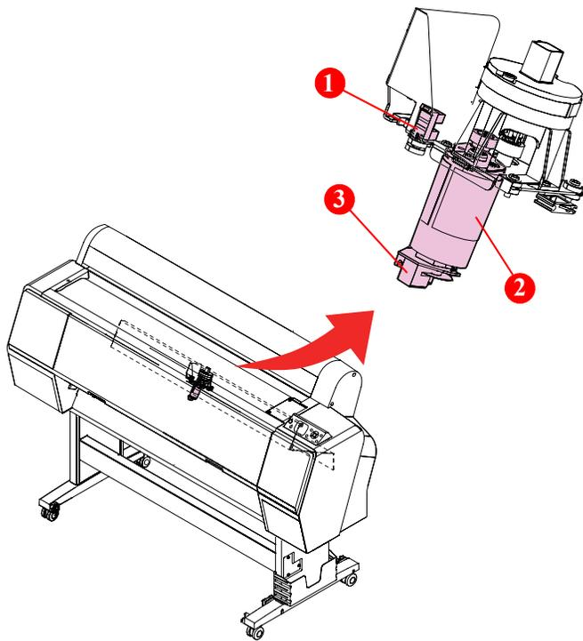
Figure 2-8. Pressurizing Unit
