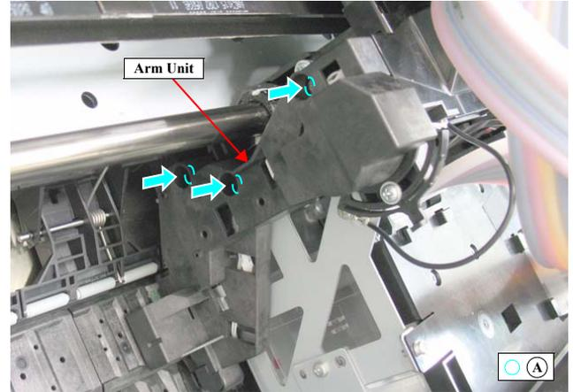
Figure 4-151. Removing the Arm Unit
