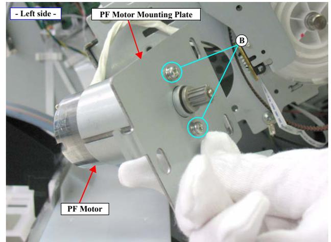
Figure 4-106. Removing the PF Motor
