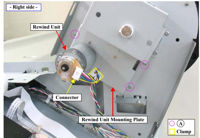
Figure 4-90. Removing the Rewind Unit Mounting Plate
