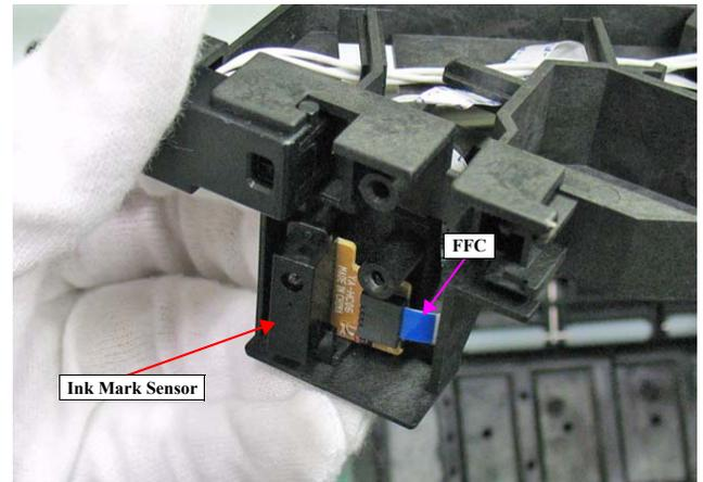
Figure 4-153. Removing the Ink Mark Sensor
