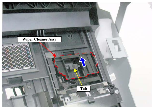
Figure 4-112. Removing the Wiper Cleaner Assy
