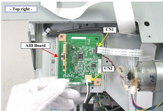
Figure 4-148. Removing the AID Board
