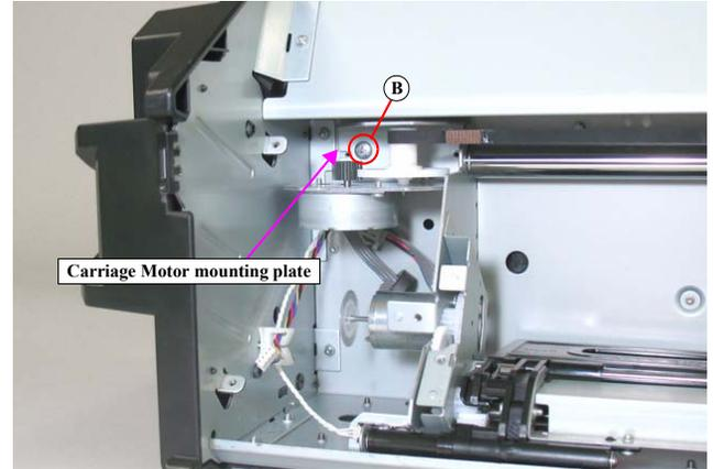
Figure 4-228. Removing the Carriage Motor mounting plate
