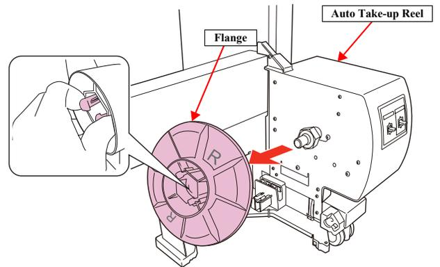
Figure 4-176. Removing the Flange
