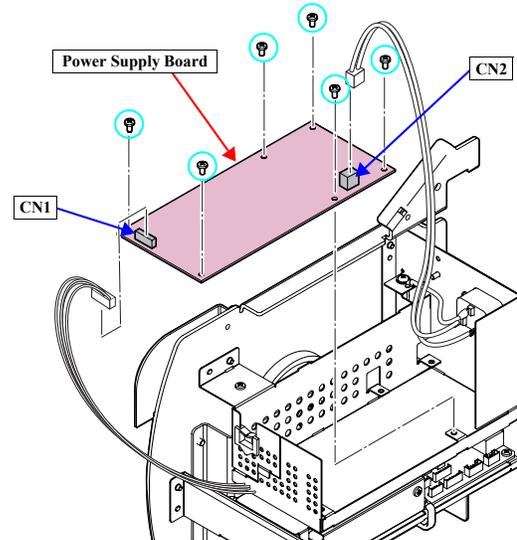
Figure 4-181. Removing the Power Supply Board
