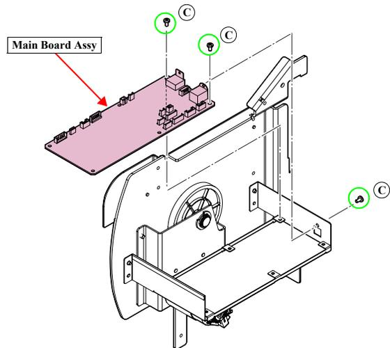
Figure 4-191. Removing the Main Board Assy
