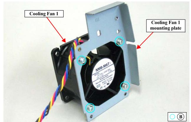
Figure 4-218. Removing the Cooling Fan 1
