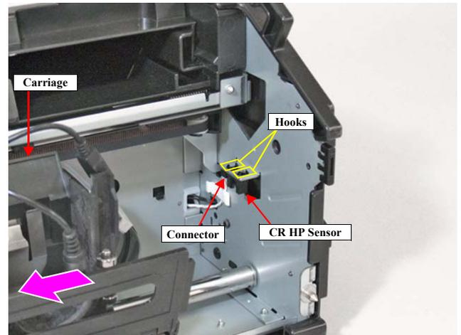
Figure 4-208. Removing the CR HP Sensor
