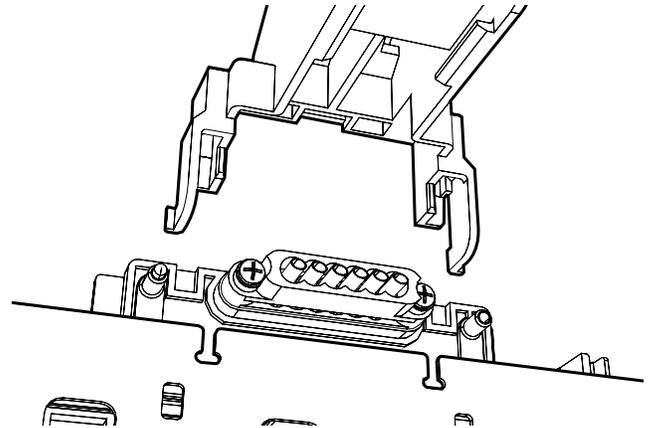
Figure 4-129. Removing the Ink Tube Guide
