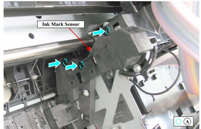
Figure 4-75. Removing the Ink Mark Sensor
