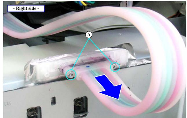
Figure 4-132. Detaching the Ink Tube
