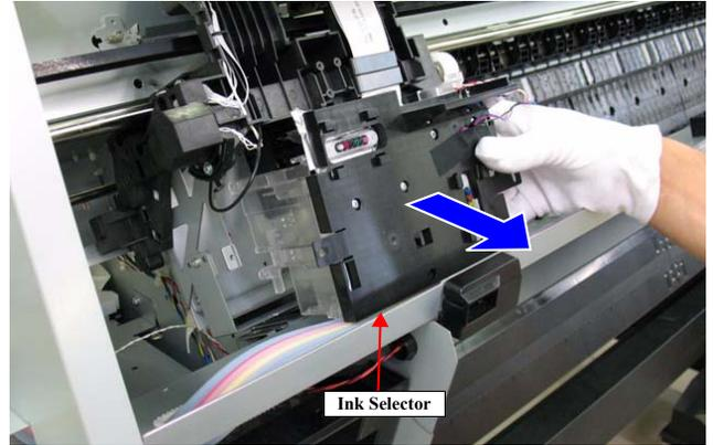
Figure 4-162. Removing the Ink Selector (2)
