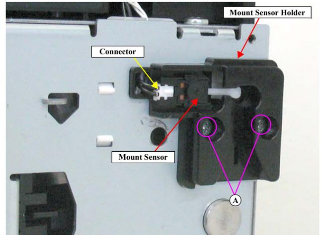
Figure 4-211. Removing the Mount Sensor
