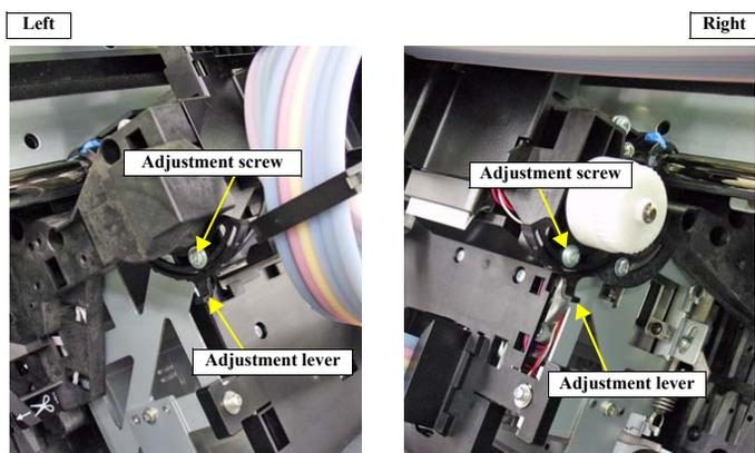
Figure 5-19. Adjustment Screw and Lever
