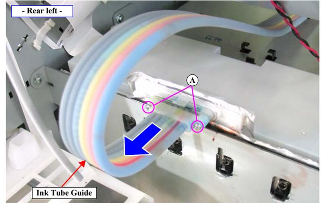
Figure 4-140. Detaching the Ink Tube
