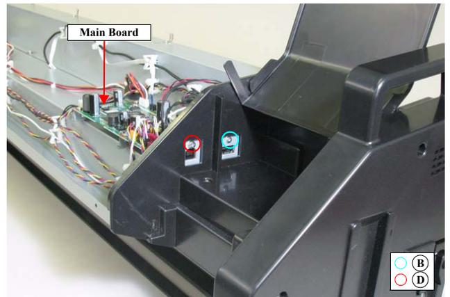
Figure 4-204. Removing the Main Board (2)
