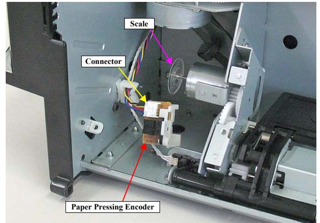
Figure 4-216. Removing the Paper Pressing Encoder
