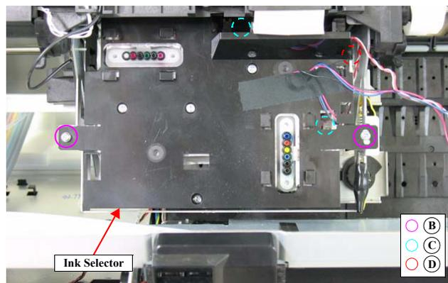
Figure 4-118. Ink Selector fixing screws (Epson Stylus Pro 7700/7710/9700/9710)
