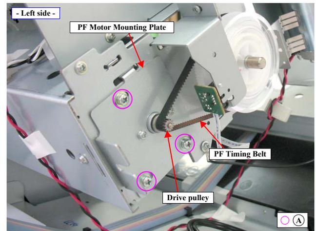
Figure 4-105. Removing the PF Motor Mounting Plate
