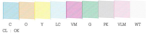
Figure 5-28. Nozzle Check Pattern (Epson Stylus Pro WT7900/WT7910)
