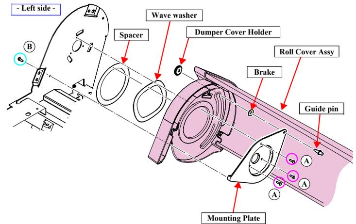
Figure 4-31. Removing the Roll Cover Assy (Left side)
