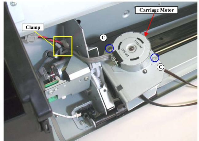
Figure 4-229. Removing the Carriage Motor
