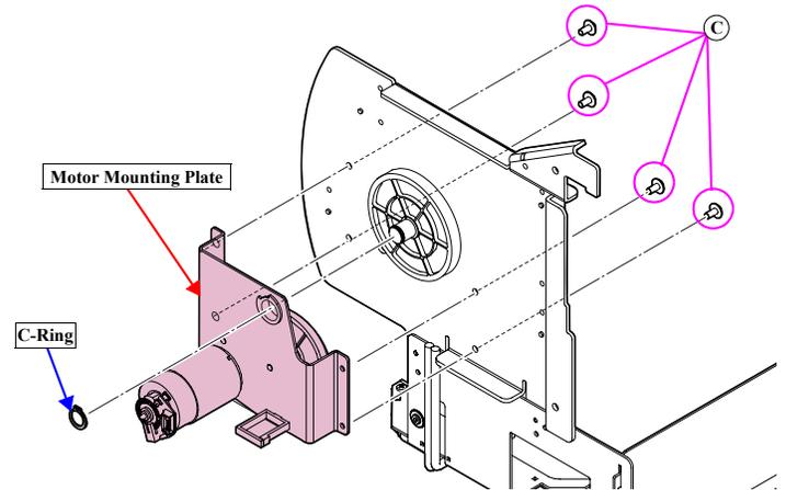
Figure 4-185. Removing the Motor Mounting Plate
