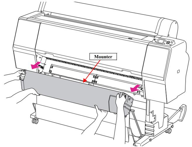
Figure 4-196. Removing the Mounter
