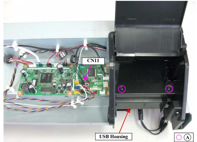
Figure 4-209. Removing the USB Housing
