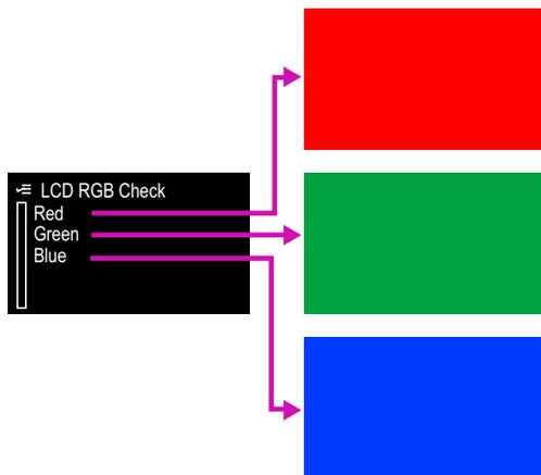
Figure 5-86. Color LCD Display Check
