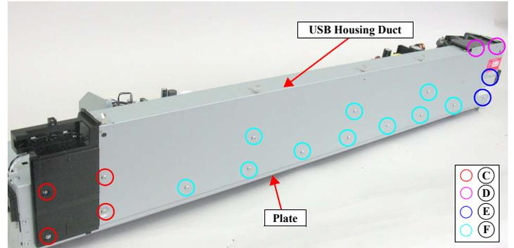
Figure 4-221. Removing the plate
