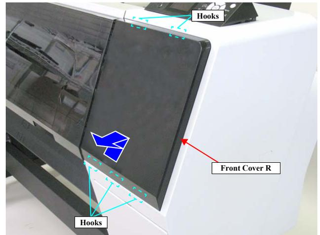
Figure 4-19. Removing the Front Cover (L/R)
