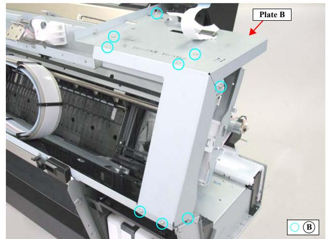
Figure 4-72. Removing the Plate B
