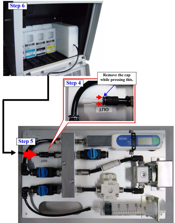
Figure 5-62. Preparation for Air Leak Check
