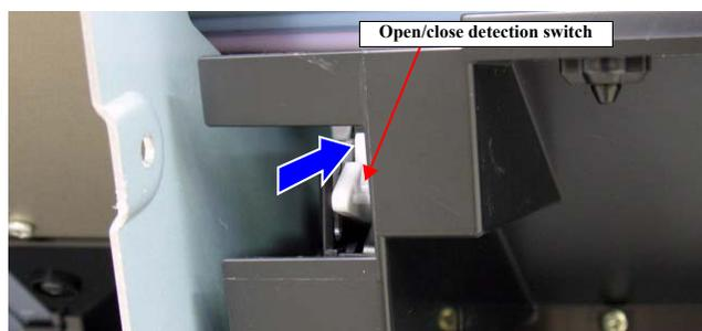
Figure 5-20. Switching the IC Cover Switch
