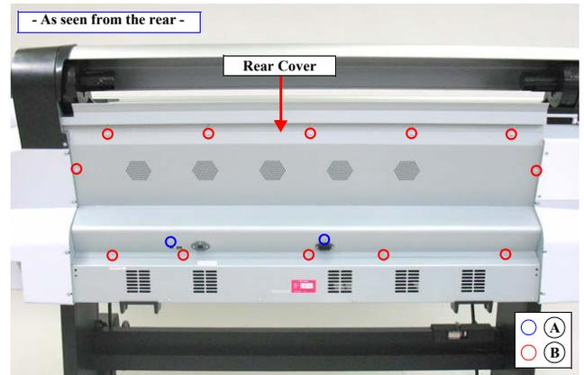
Figure 4-35. Removing the Rear Cover
