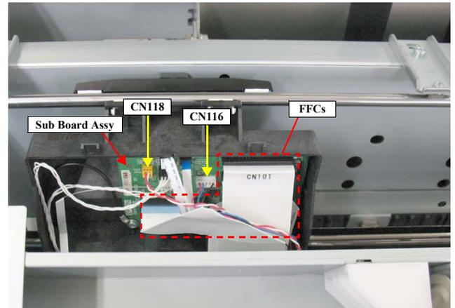
Figure 4-114. Disconnecting the connectors
