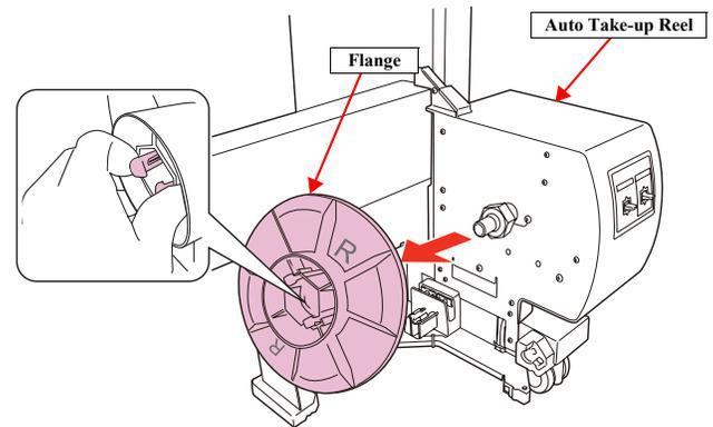
Figure 4-179. Removing the Flange
