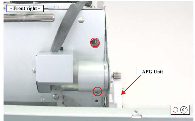
Figure 4-73. Removing the APG Unit
