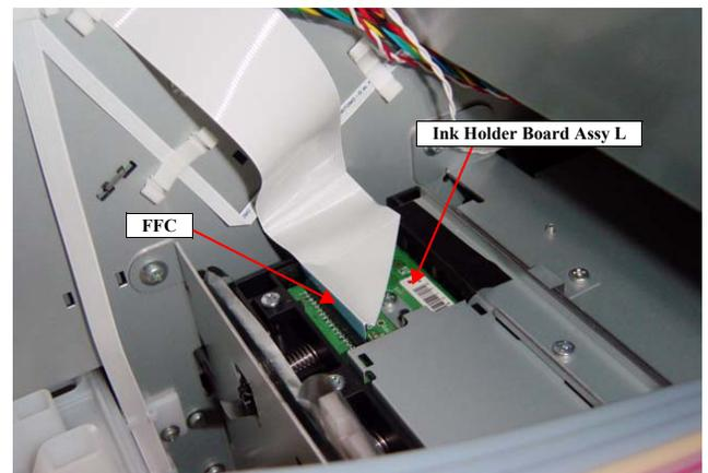
Figure 4-139. Disconnecting the FFC
