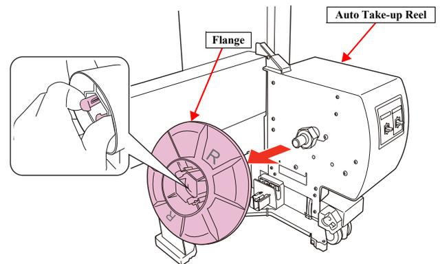
Figure 4-187. Removing the Flange
