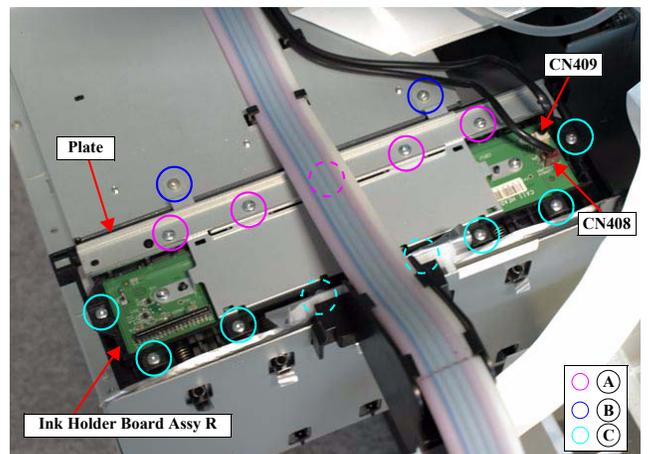
Figure 4-146. Removing the Ink Holder Board Assy R
