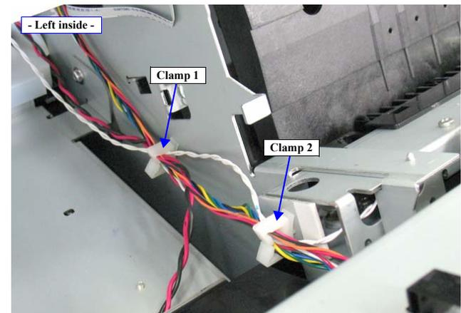
Figure 4-97. Releasing the Harness
