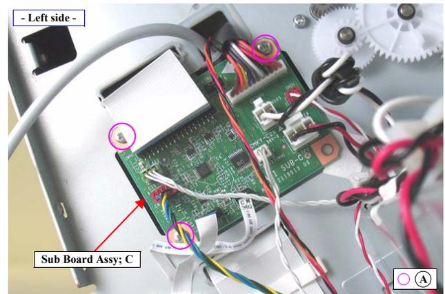
Figure 4-57. Removing the Sub Board Assy; C
