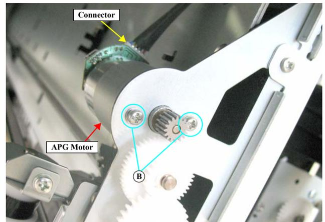
Figure 4-70. Removing the APG Motor (2)
