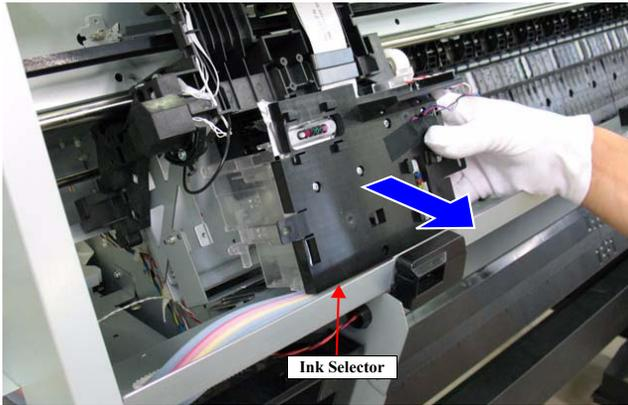
Figure 4-119. Removing the Ink Selector
