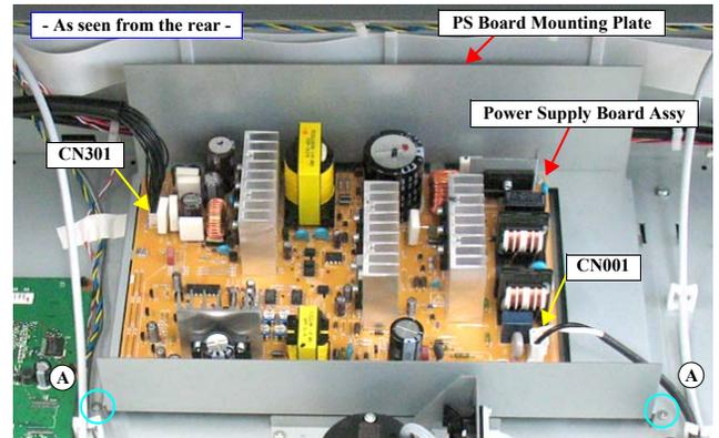
Figure 4-49. Removing the PS Board Mounting Plate
