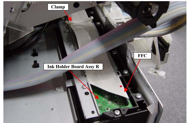
Figure 4-131. Disconnecting the FFC
