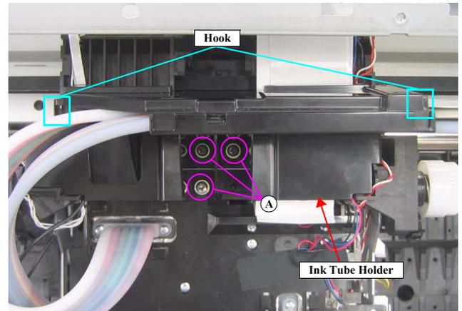
Figure 4-156. Removing the Ink Tube Holder
