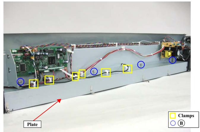
Figure 4-220. Releasing the harnesses
