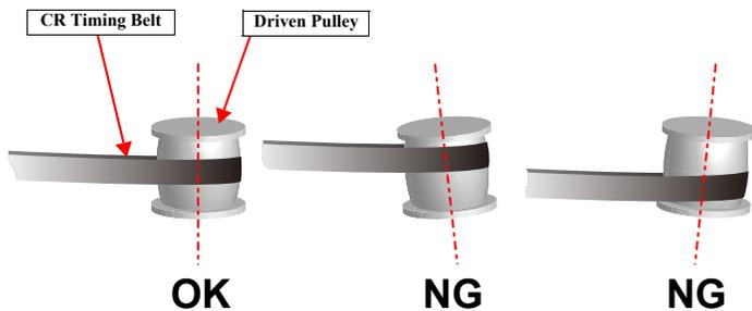
Figure 5-12. Slant Adjustment of Driven Pulley
