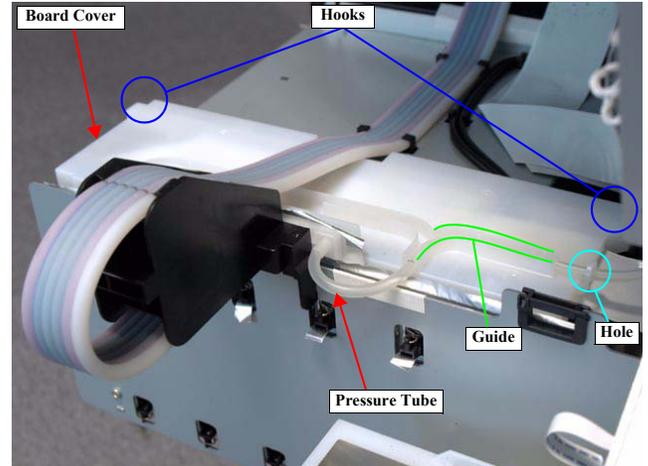
Figure 4-144. Removing the Board Cover
