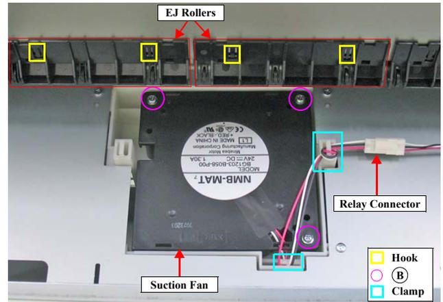
Figure 4-101. Removing the Suction Fan
