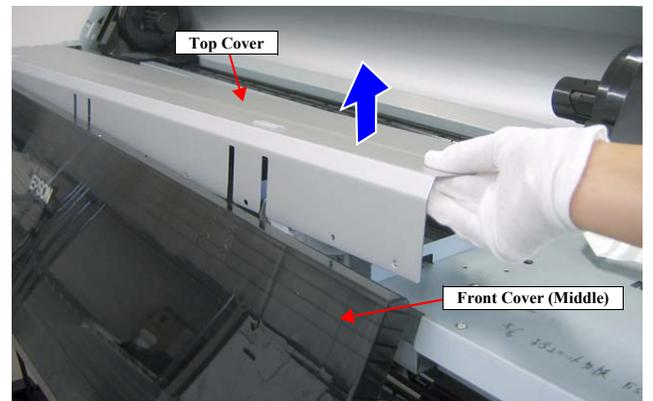
Figure 4-27. Removing the Top Cover (2)
