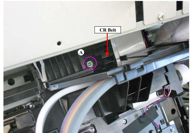
Figure 4-63. Removing the CR Belt
