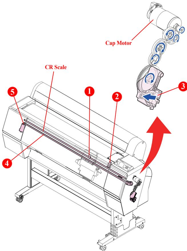
Figure 2-3. Carriage Mechanism
