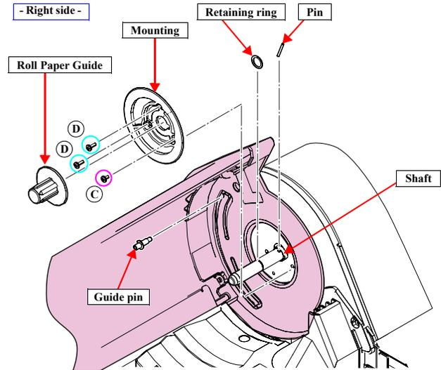
Figure 4-32. Removing the Roll Cover Assy (Right side)
