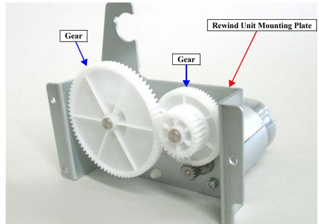
Figure 4-91. Removing the gears
