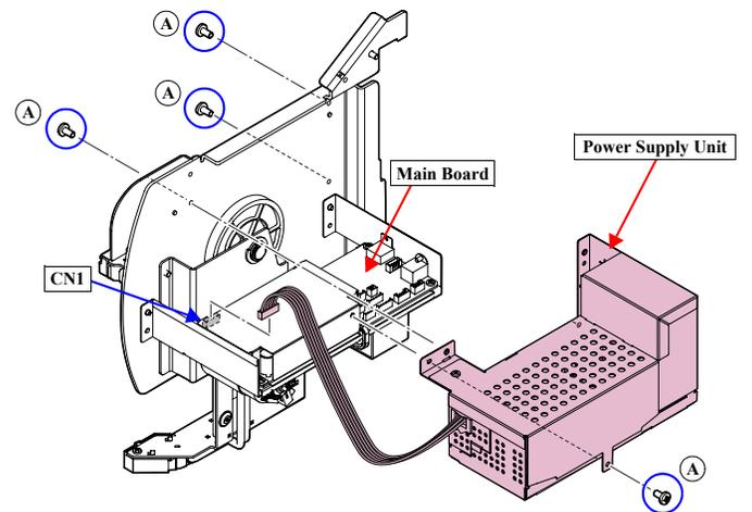
Figure 4-177. Removing the Power Supply Unit
