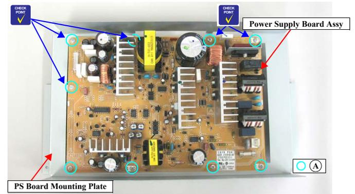
Figure 4-50. Removing the Power Supply Board Assy
