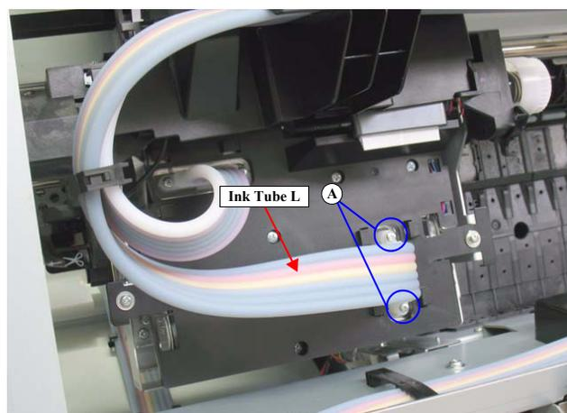
Figure 4-169. Removing the Ink Tube L
