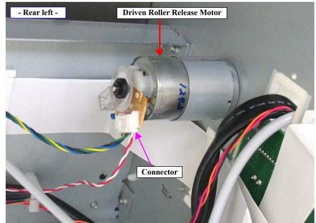
Figure 4-87. Disconnecting the connector
