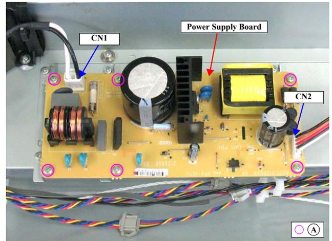
Figure 4-205. Removing the Power Supply Board
