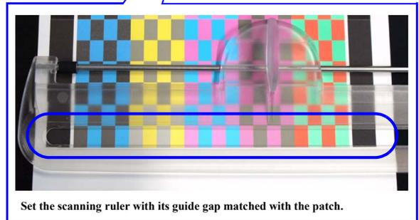
Set the scanning ruler with its guide gap matched with the patch.
