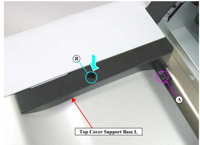
Figure 4-23. Removing the Top Cover Support Base L
