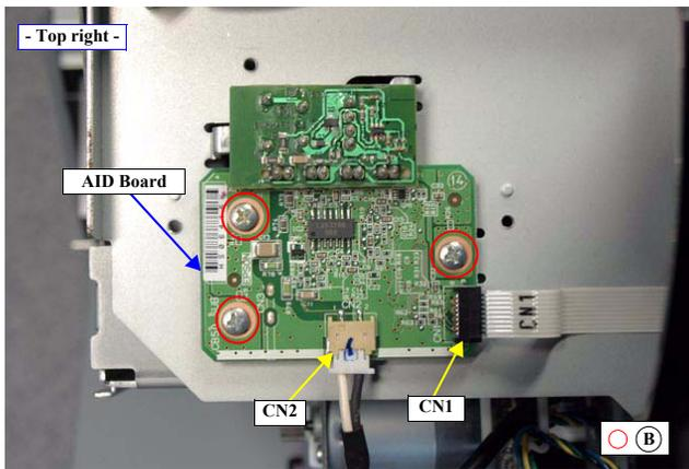
Figure 4-150. Removing the AID Board
