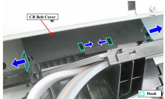
Figure 4-62. Removing the CR Belt Cover
