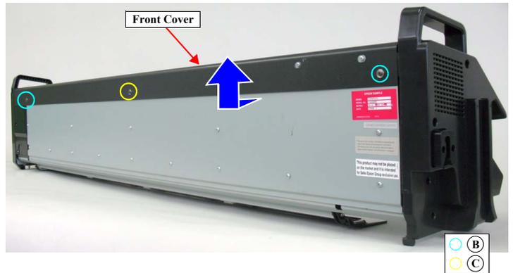
Figure 4-201. Removing the Front Cover (2)
