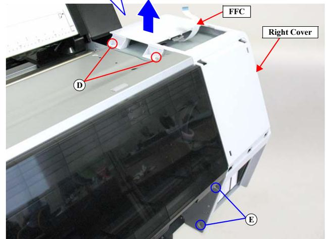
Figure 4-22. Removing the Right Cover
