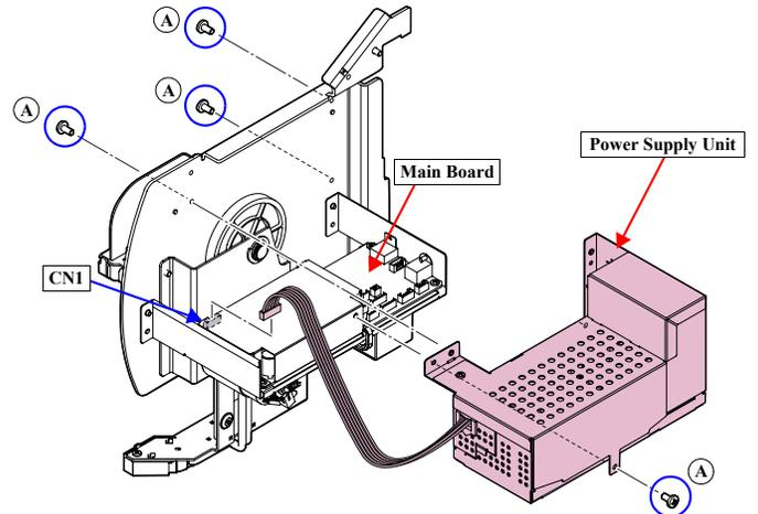
Figure 4-174. Removing the Power Supply Unit
