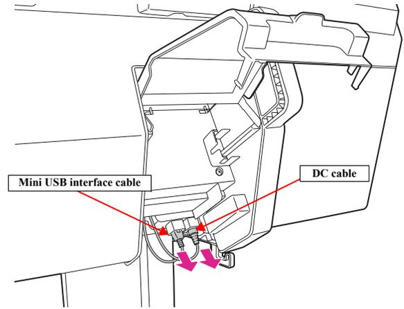
Figure 4-194. Disconnecting the cables (2)
