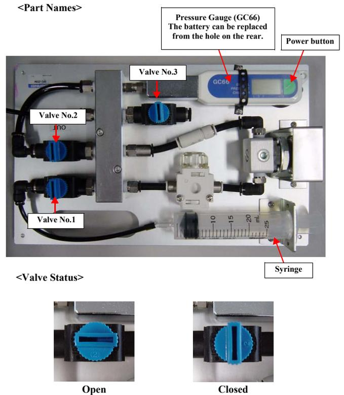
Figure 5-63. Operation of the Ink Leak Measurement Jig
