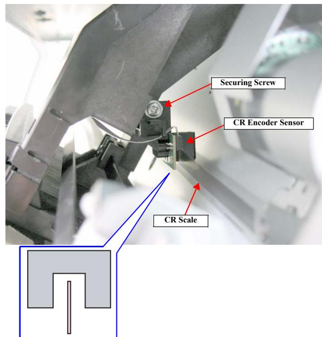
Figure 5-17. CR Encoder Sensor Adjustment
