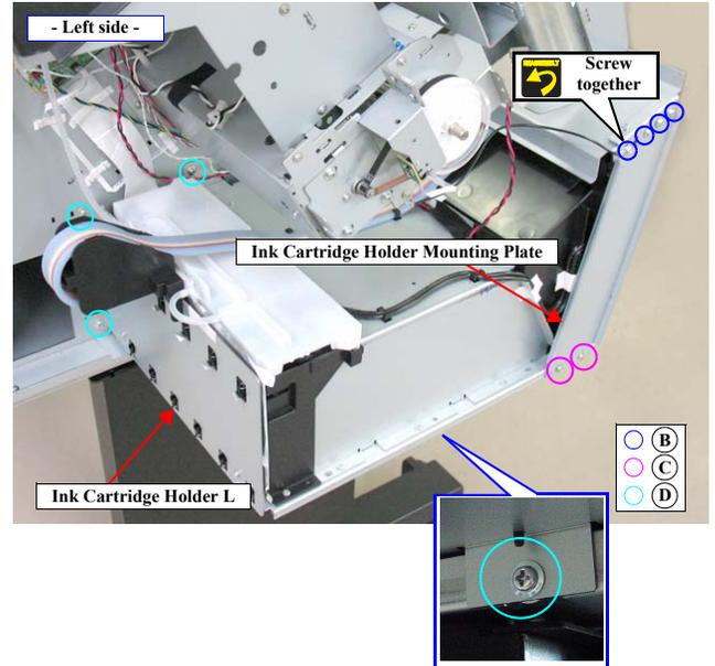
Figure 4-141. Removing the Ink Cartridge Holder L
