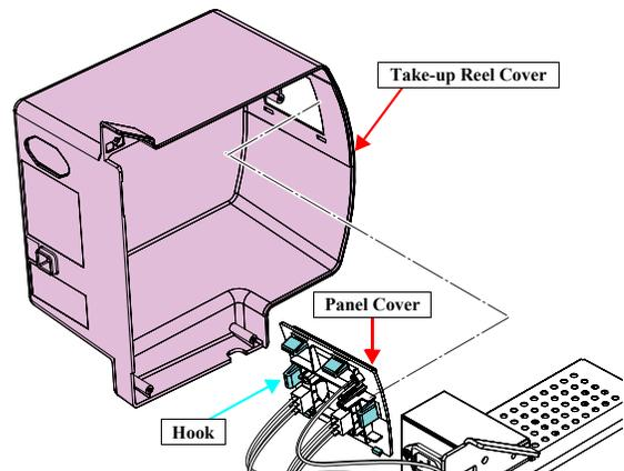
Figure 4-171. Removing the Take-up Reel Cover
