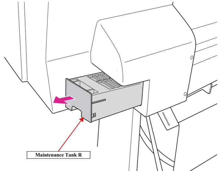
Figure 4-20. Removing the Maintenance Tank (L/R)
