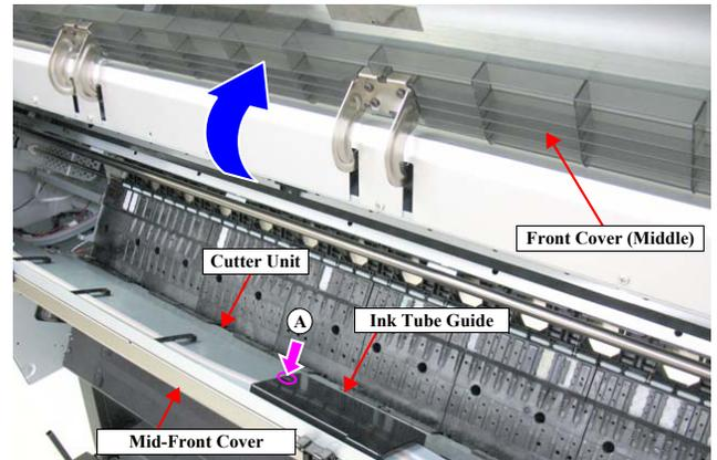
Figure 4-93. Removing the Ink Tube Guide
