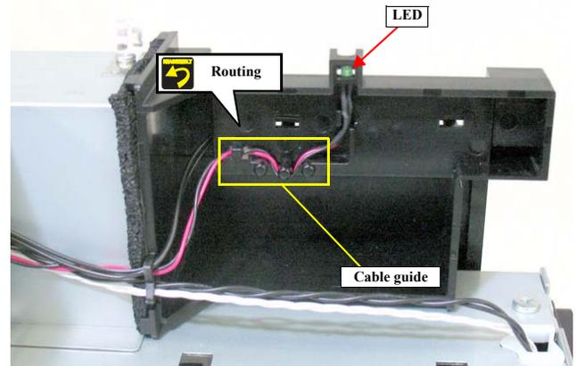
Figure 4-213. Removing the LED
