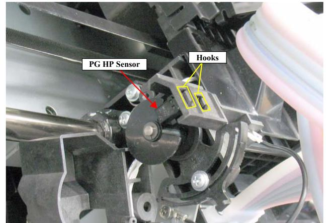
Figure 4-77. Removing the PG HP Sensor (1)
