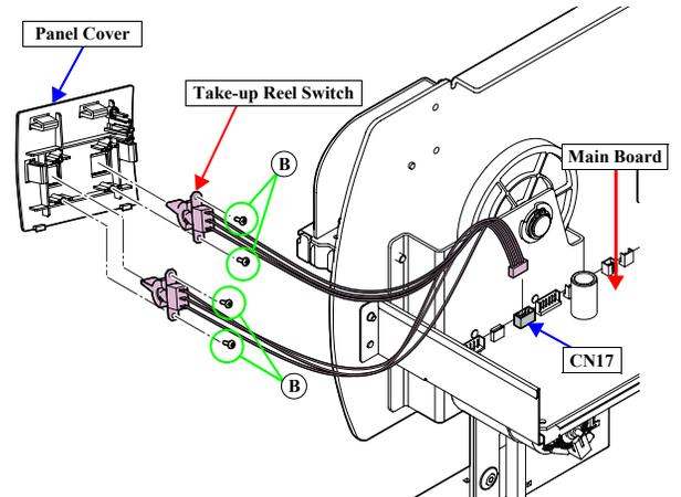
Figure 4-178. Removing the Take-up Reel Switch
