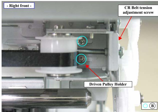
Figure 4-64. Removing the Driven Pulley Holder
