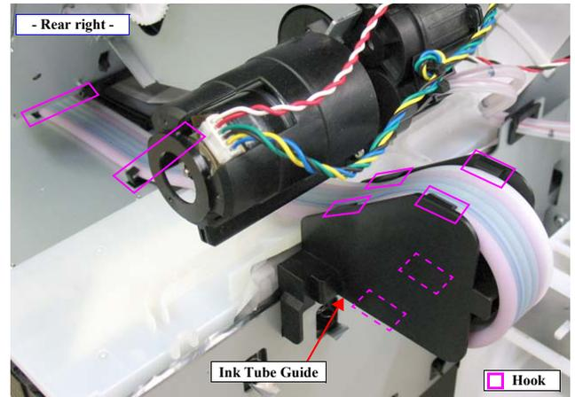
Figure 4-126. Releasing the Ink Tube Guide (before released)
