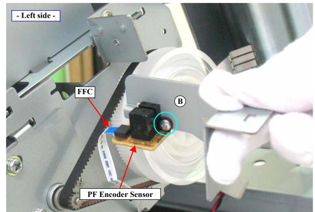
Figure 4-103. Removing the PF Encoder Sensor
