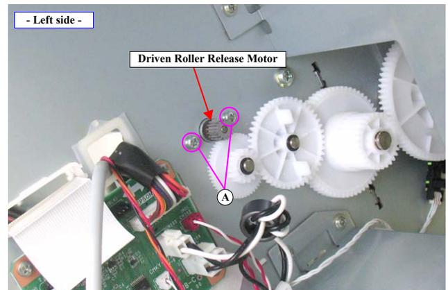
Figure 4-88. Removing the Driven Roller Release Motor
