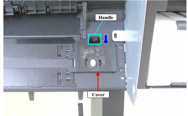
Figure 4-99. Removing the cover
