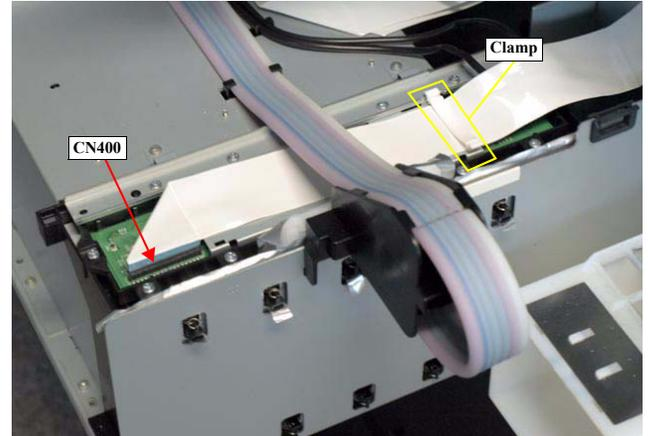
Figure 4-145. Releasing the FFC
