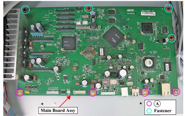
Figure 4-48. Removing the Main Board Assy
