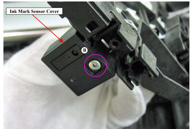
Figure 4-152. Removing the Ink Mark sensor Cover
