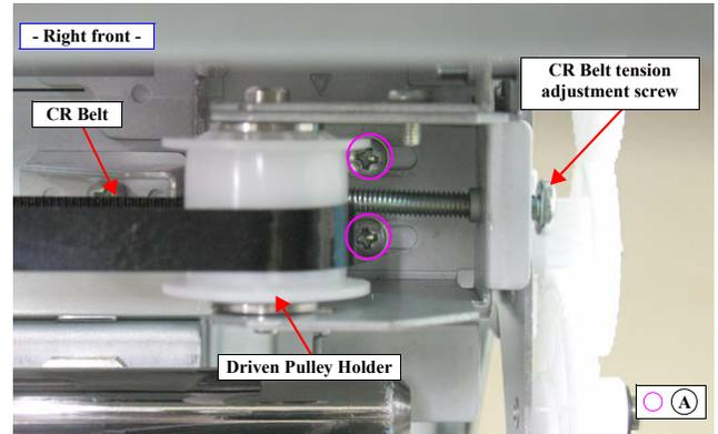
Figure 4-67. Relieving the tension of the CR Belt
