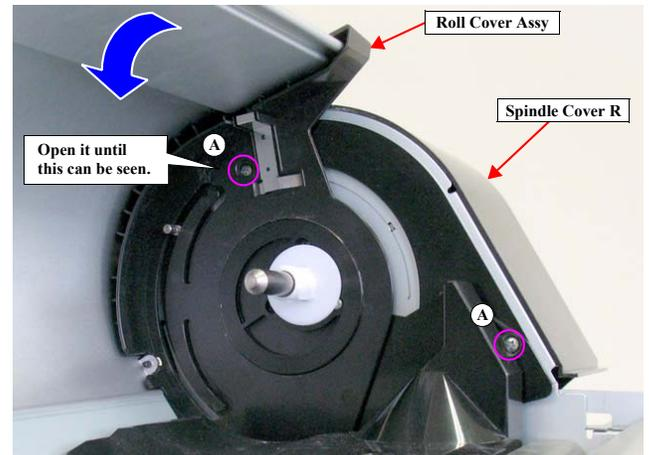
Figure 4-28. Removing the screws (inside)
