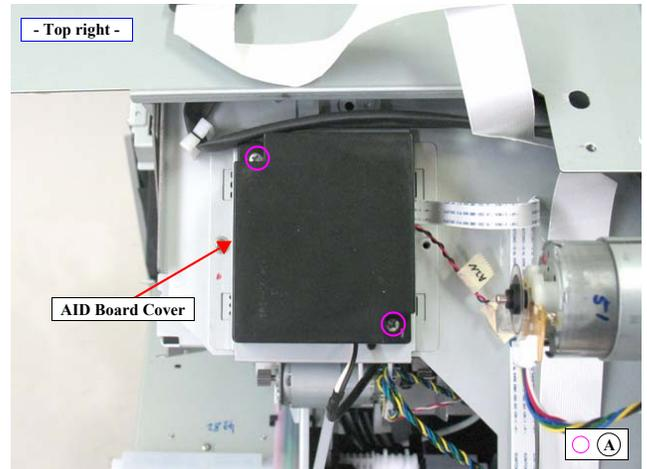
Figure 4-109. Removing the AID Board Cover
