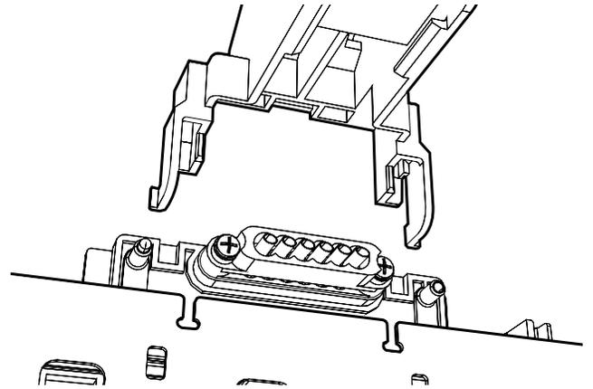
Figure 4-137. Removing the Ink Tube Guide
