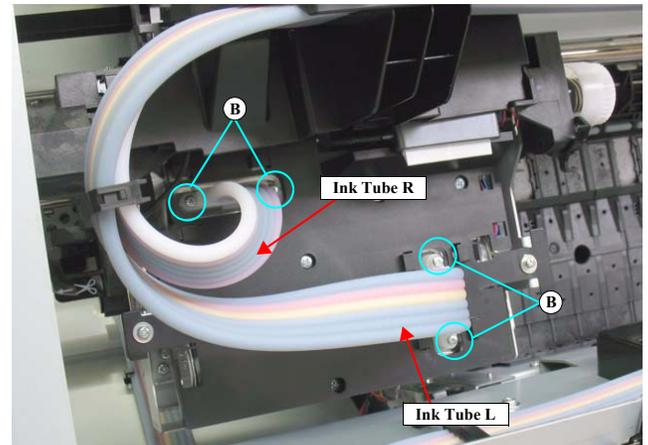
Figure 4-159. Removing the Ink Tube L and R
