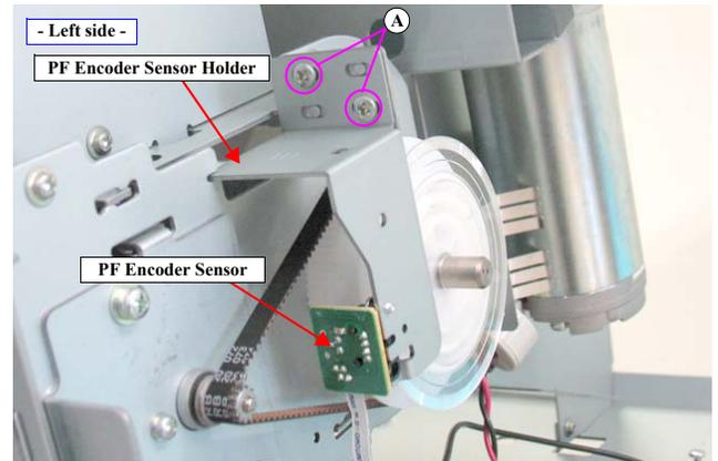
Figure 4-102. Removing the PF Encoder Sensor Holder
