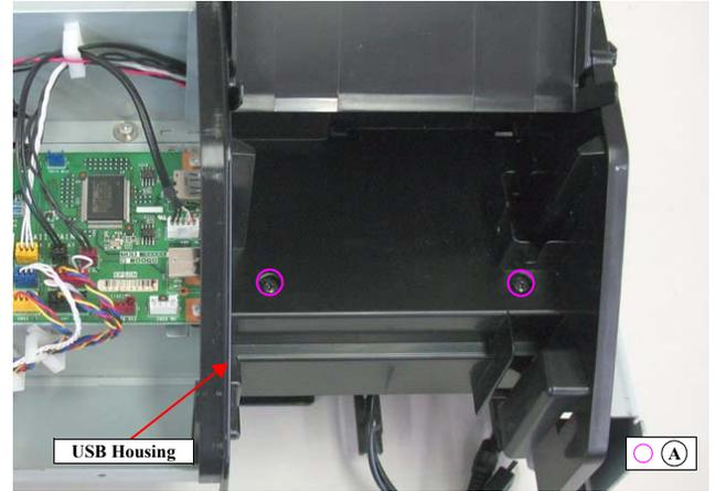
Figure 4-219. Removing the USB Housing
