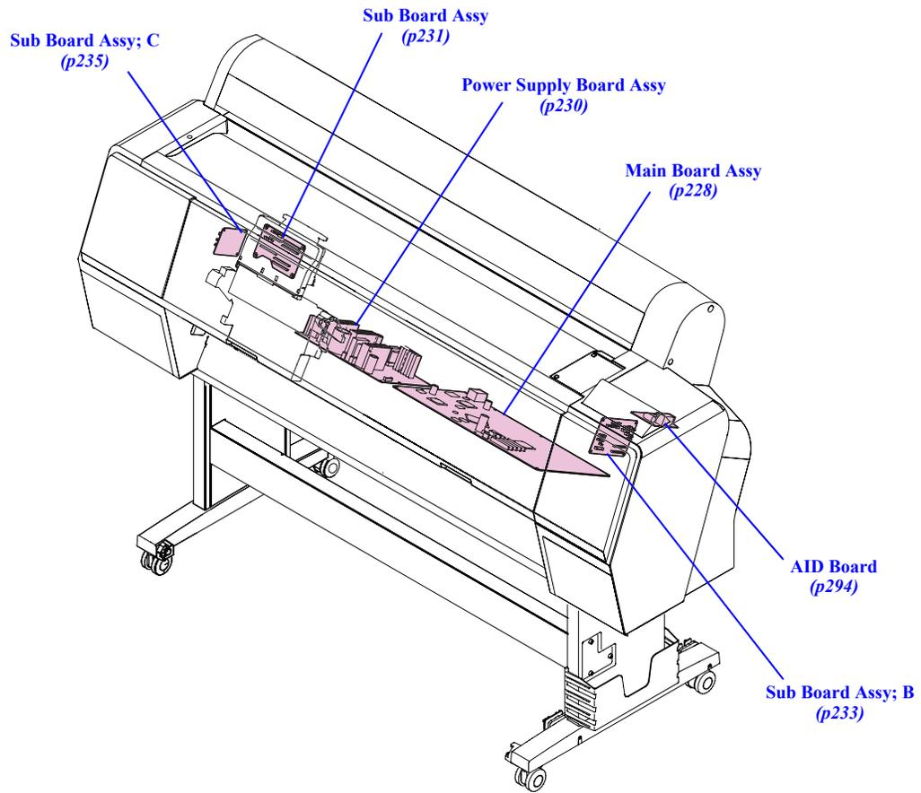
Figure 4-6. Electric Circuit Components
