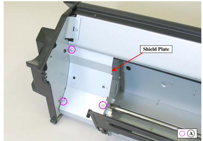
Figure 4-226. Removing the shield Plate
