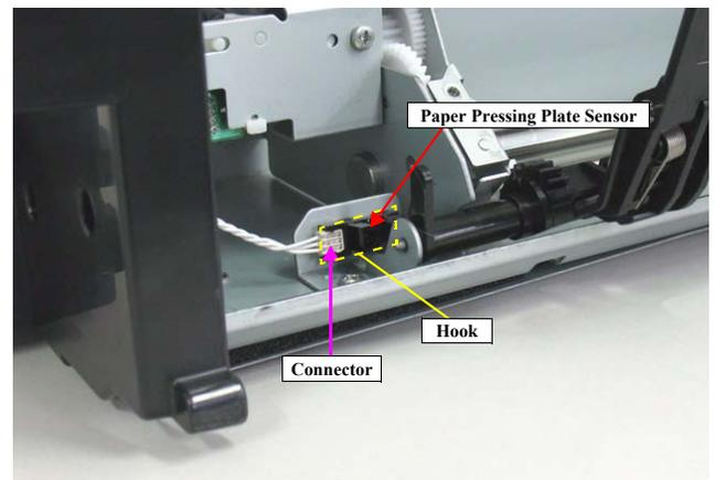
Figure 4-207. Removing the Paper Pressing Plate Sensor
