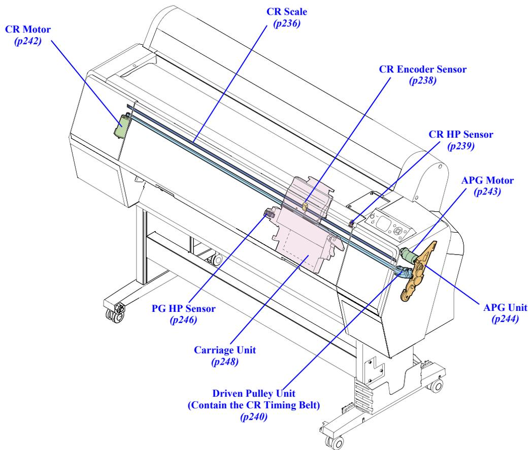
Figure 4-7. Carriage Mechanism
