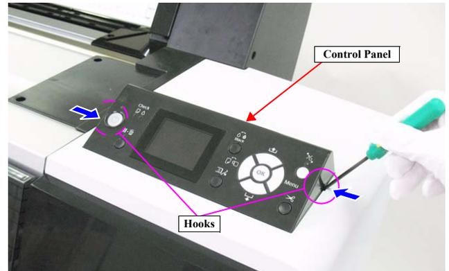
Figure 4-14. Removing the Control Panel
