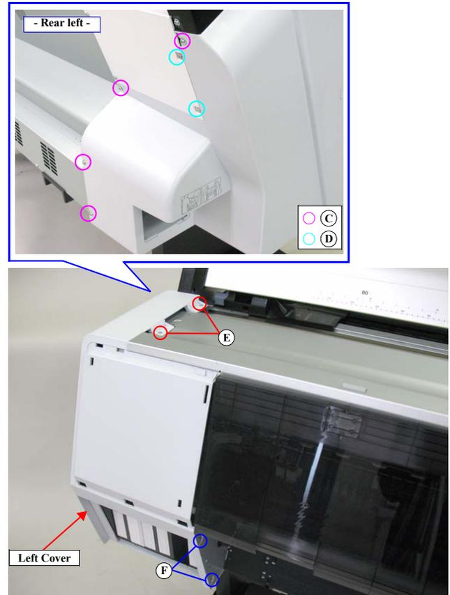
Figure 4-24. Removing the Left Cover
