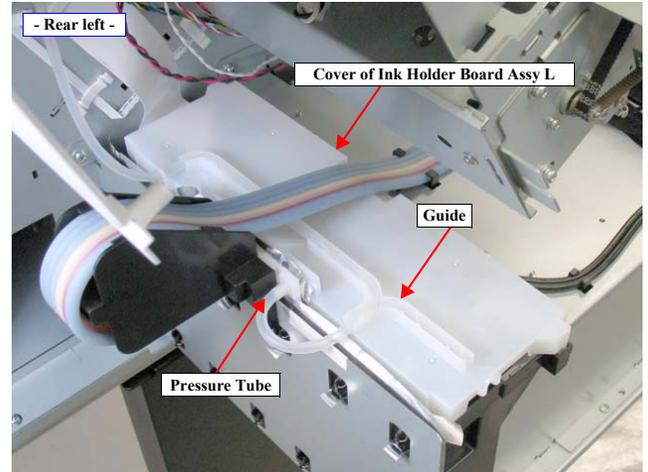
Figure 4-44. Releasing the Pressure Tube
