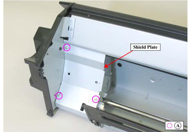
Figure 4-214. Removing the shield Plate
