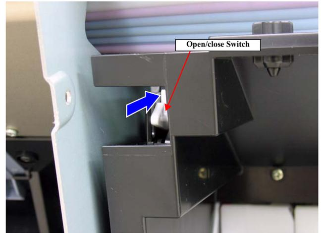
Figure 5-11. Switching the IC cover mode
