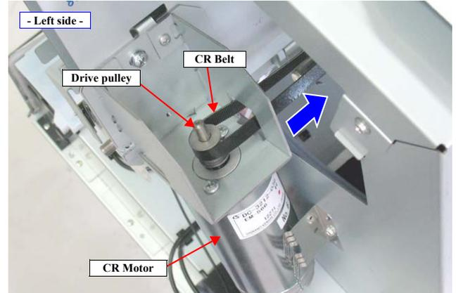
Figure 4-65. Removing the CR Belt
