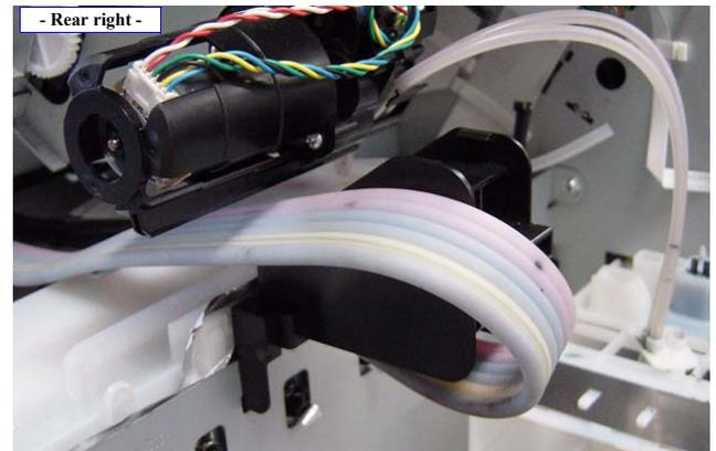
Figure 4-127. Releasing the Ink Tube Guide (after released)
