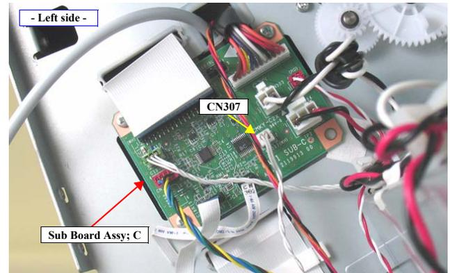
Figure 4-96. Disconnecting the connector
