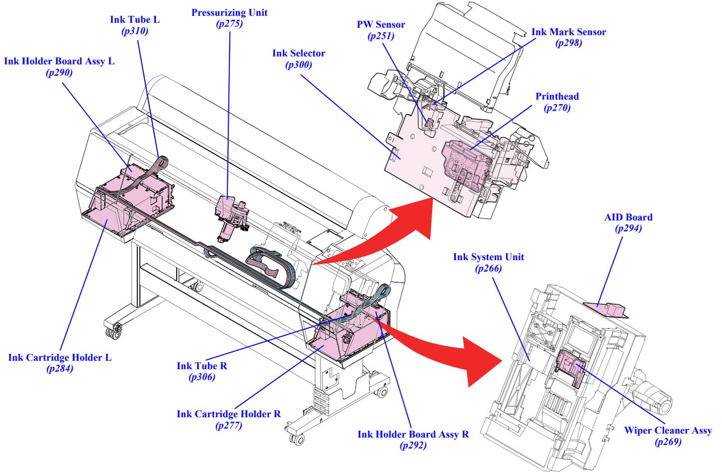
Figure 4-9. Ink System Mechanism
