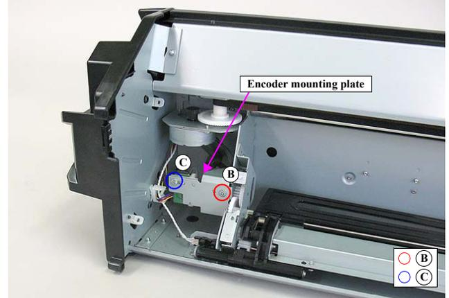
Figure 4-215. Removing the encoder mounting plate
