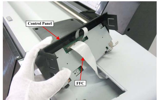
Figure 4-15. Disconnecting the FFC
