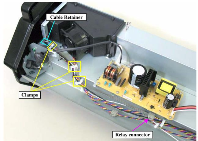
Figure 4-227. Disconnecting the relay connector
