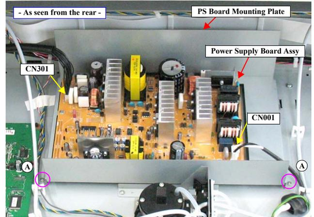
Figure 4-39. Removing the PS Board Mounting Plate
