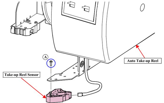
Figure 4-172. Removing the Take-up Reel Sensor
