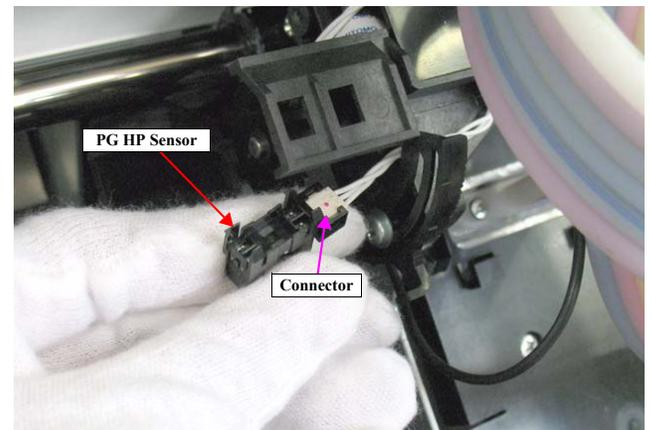
Figure 4-78. Removing the PG HP Sensor (2)
