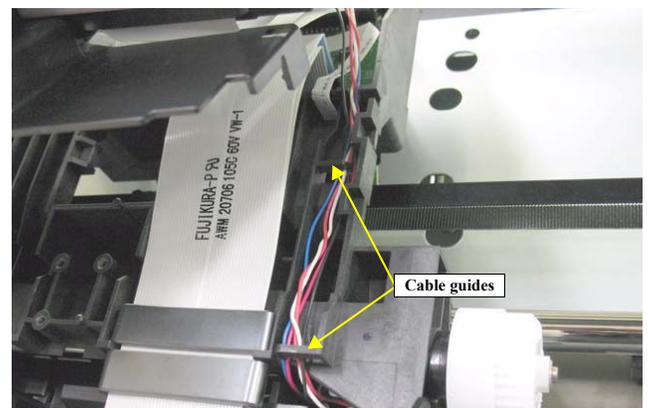
Figure 4-157. Releasing the Harness
