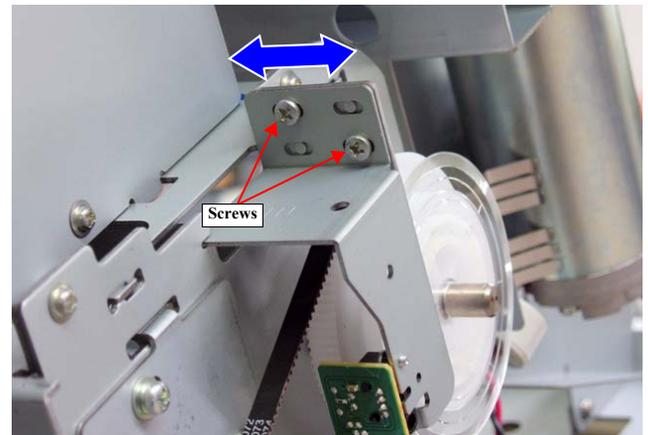
Figure 5-72. PF Encoder Sensor Adjustment
