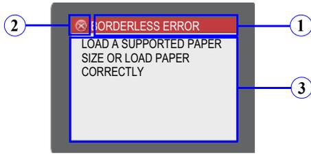
Figure 1-10. LCD (Error indication)
