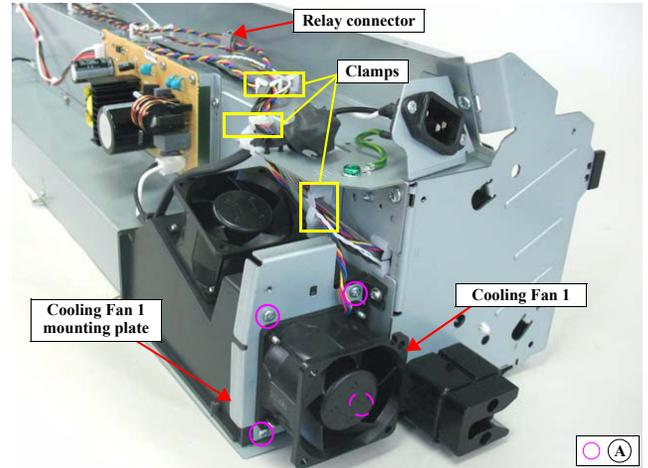
Figure 4-217. Removing the Cooling Fan 1 mounting plate
