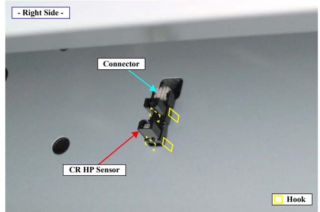
Figure 4-61. Removing the CR HP Sensor
