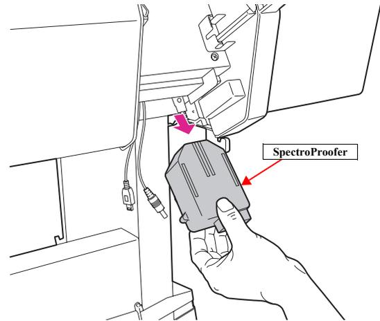
Figure 4-195. Removing the Color Measurement Device
