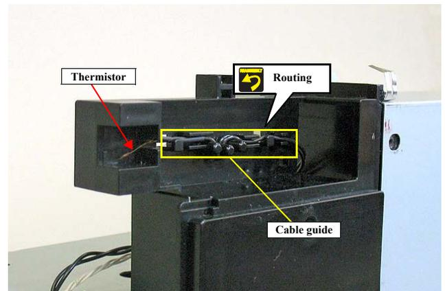
Figure 4-210. Removing the Thermistor
