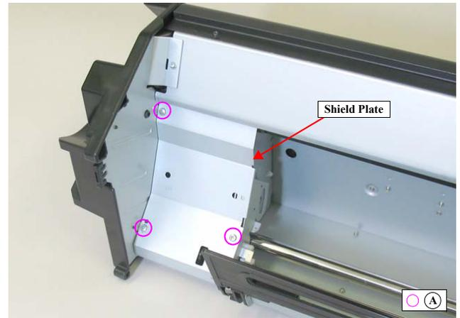
Figure 4-230. Removing the shield Plate
