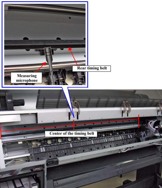
Figure 5-15. Measuring the Timing Belt Tension
