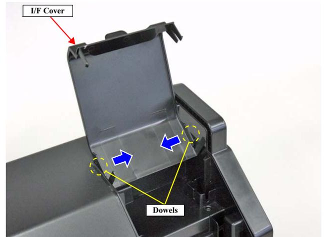
Figure 4-199. Removing the I/F Cover
