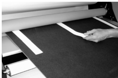
2. check pressure with strips of paper.
