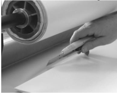
5. cut off starter sled in back of laminator.
