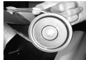
4. install belt on pulleys
