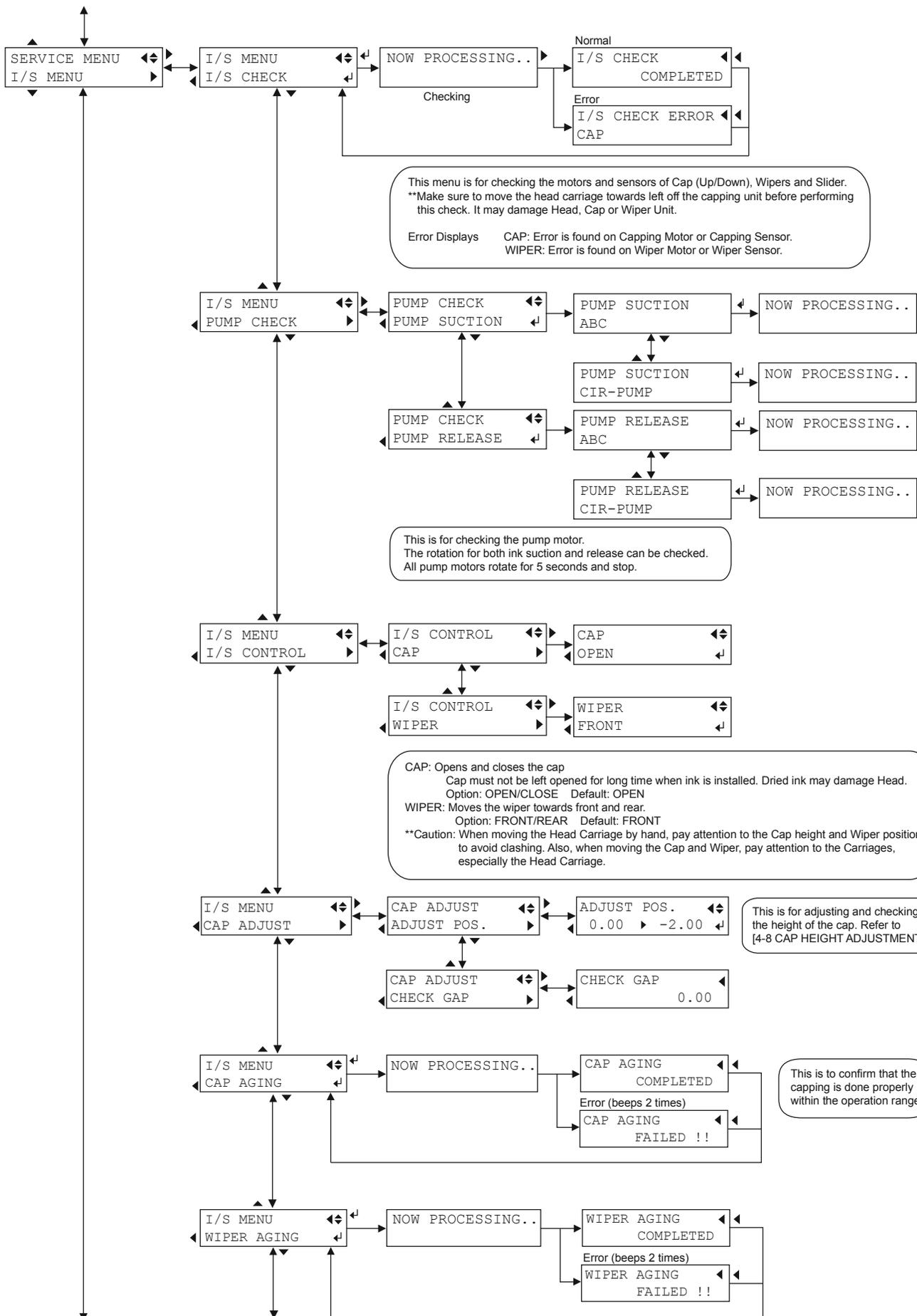
This menu is for checking the motors and sensors of Cap (Up/Down), Wipers and Slider.
