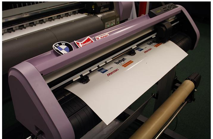
5. Use arrow keys to jog LED light to correct position for mark detection using following guide and press “Enter” to detect the registration marks
