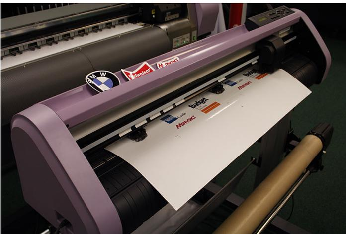
4. Use arrow keys to jog LED light to correct position for mark detection using following guide and press “Enter” to detect the registration marks
