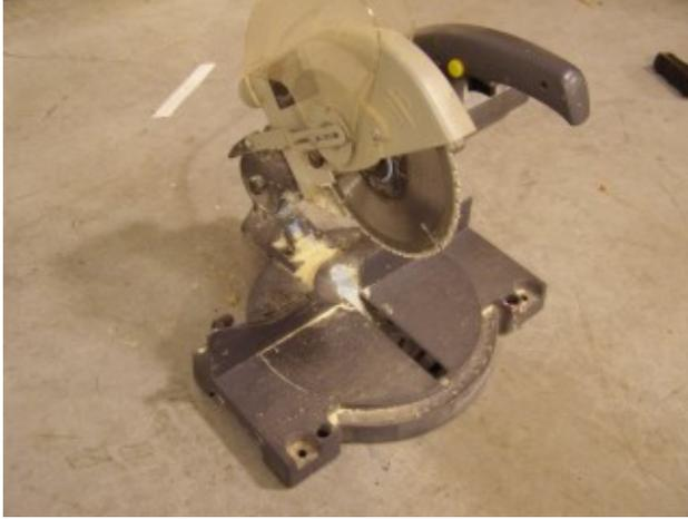
Cutting down vinyl rolls to size.....yes it can be done! With good results. With the following pics it's self explanatory...here I cut down a 54" x 10 Yard roll of LG 3910. The saw - cheapo Sears Craftsman 7 1/4 well over 10 years old. The blade is similar to this [one](#). I also have a 12" out on loan right now(where is my saw BOB?)...I use for bigger rolls.
