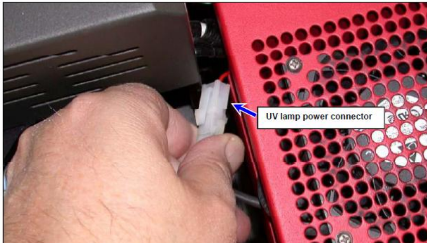
Figure 2: UV Lamp Power Connections
