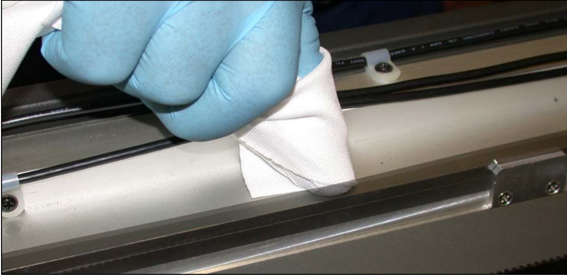
Figure 54 Cleaning the Optical Encoder Strip
