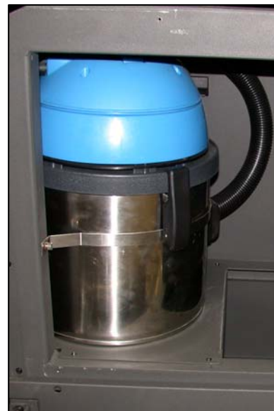
Replace vacuum body filter per maintenance schedule
