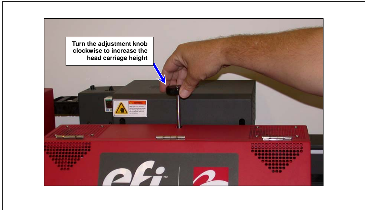
Figure 29 Adjusting the Head Carriage Height
