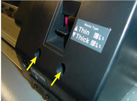
1-1. Ensure both power switches are off. Move Carriage out over Platen by hand. Remove indicated screws and remove Head Cover.
