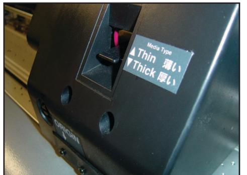
4-8. With Carriage out over the Platen, fully tighten the hex screws that secure the Print Head. Replace the Head Cover and press END several times to return to LOCAL mode.
