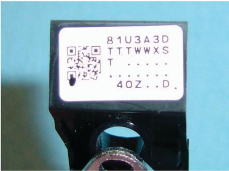
2-1. Unpackage new head. Copy down the new Head ID exactly as it appears on head.
