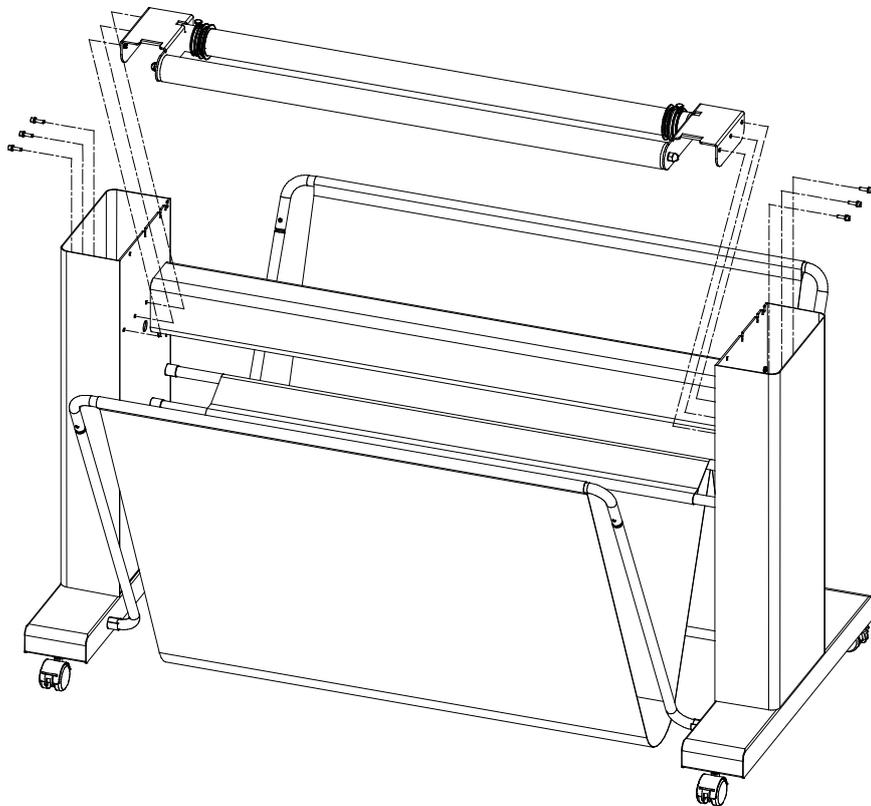
6. Remove protective paper from tape and mount sensor roll-up system 370mm from the side.
