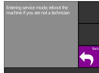
1. Switch on the cutter while pressing in the upper left corner of the touch screen.
