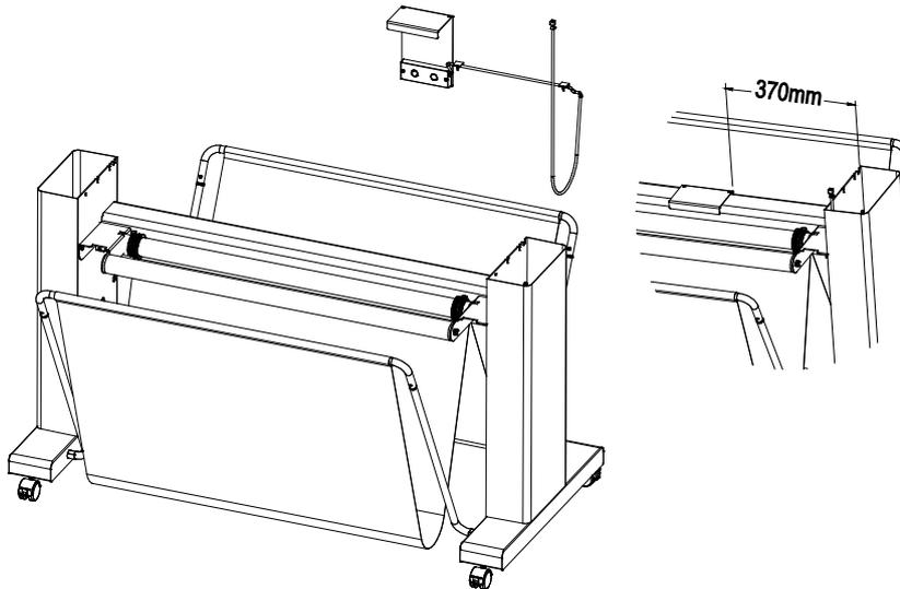
7. Fix cables to the horizontal bar with cable tie feet and cable ties. Then guide the cables through the hole in the stand and put cable protection over it.
