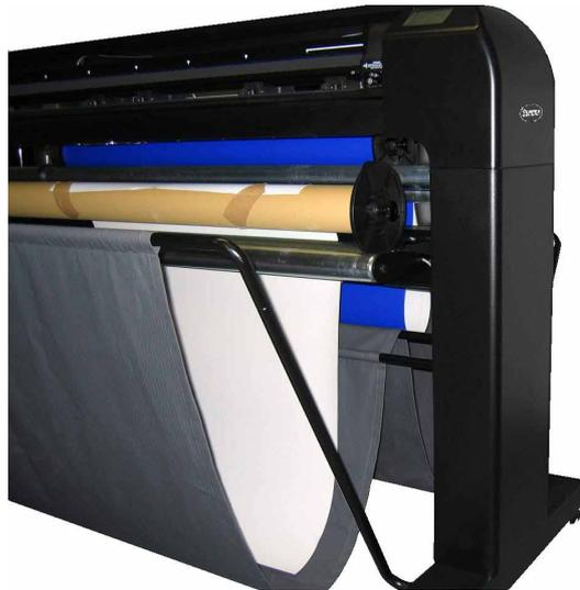
3. Attach the piece of scrap to the loaded media. It is recommended to advance the media a couple of cm, or to cut first a small job so the scrap media does not get caught when media is fed back and forth.
