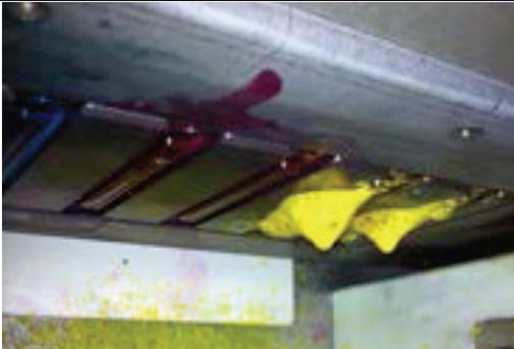
Figure 2: Foam on Printhead Nozzle Plates
