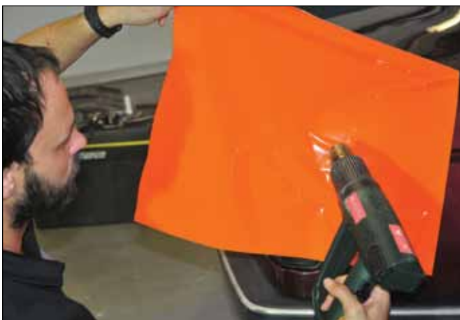
Normally, the film covering the corner is heated up.
