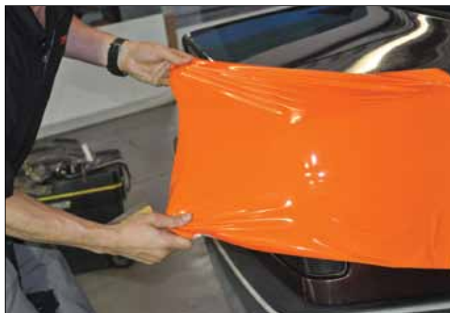
It is then pulled onto the corner.
