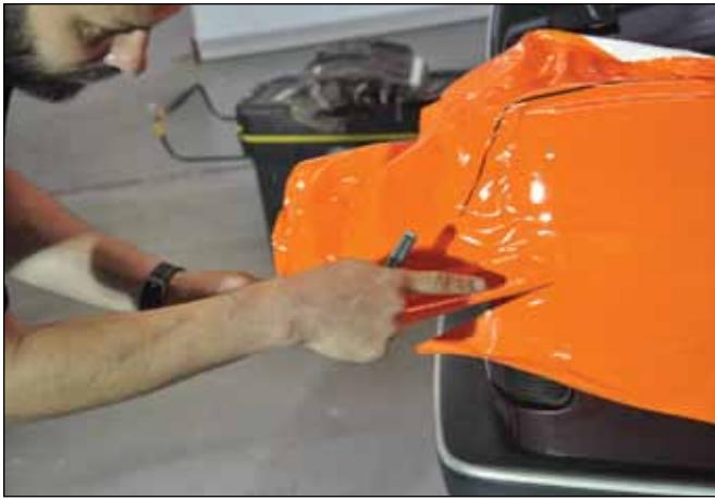
Making well-placed relief cuts lets the film wrap onto the corner with less tension.
