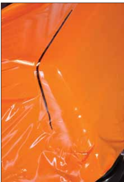
The black line marks the edge where the overstretched film is normally cut off.
