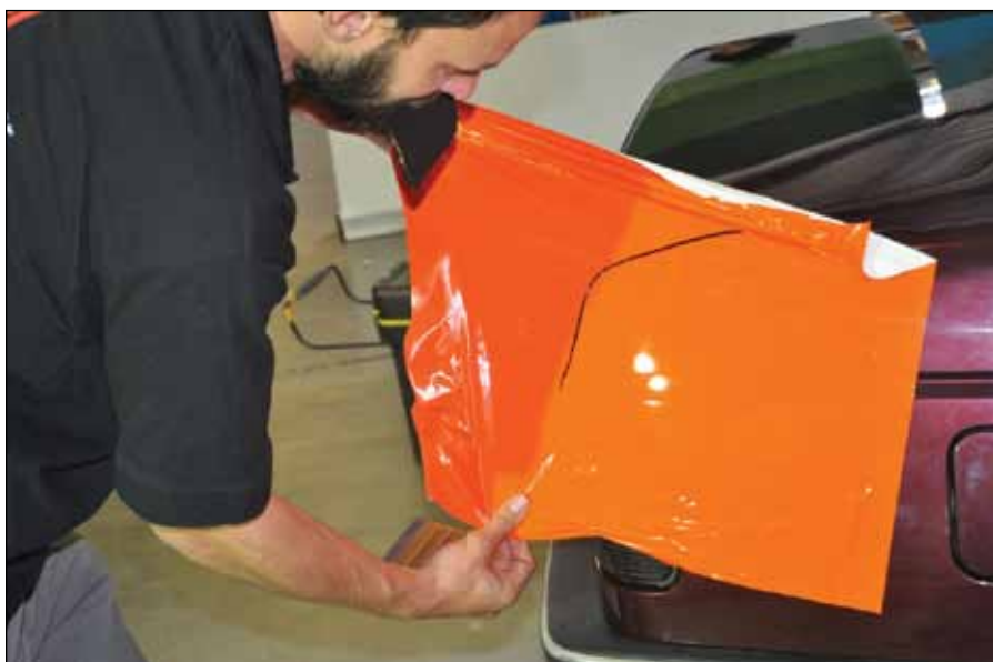
Now the piece is re-installed using sound technique, relief cuts and the right buffers on the squeegee.
