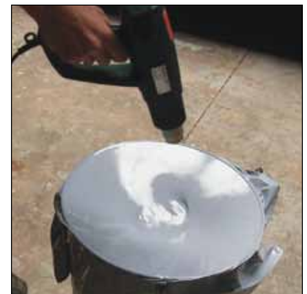
I do this to show how flexible and strong today's films are. The chemical and physical properties of PVC give the film memory. I tell the people in my workshops that this memory is both your friend and enemy because as helpful as it is, it gives many installers the impression that you can do just about anything with the vinyl.
