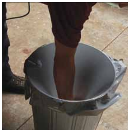
I heat the film up and push my fist down into the film, stretching it dramatically.
