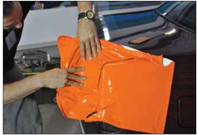
Pulling with wide fingers and making micro-adjustments allows the corner to be wrapped with no heat.
