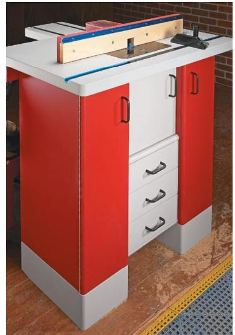
▲ **Fully Enclosed.** Adding a door and back panel to the ultimate router table helps contain dust and reduce noise.
