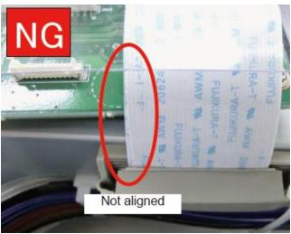
**3.** Correct the alignment if need be by unclamping the cables and resetting them. You can use masking tape to help align the cables.
