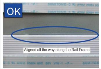
**9.** Check to make sure the outermost cable is aligned to the 3 long ribbon cables all along the rail frame.
