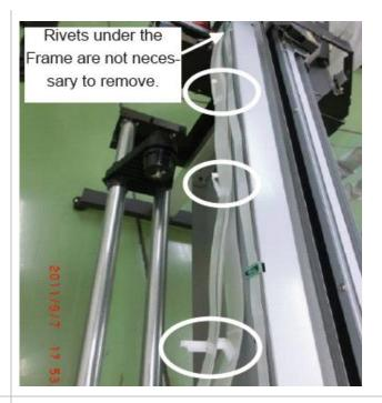
**16.** From the window in the picture pull the length of cable needed so the clear insulation cable can pass through the green board in steps 13 and 14.
