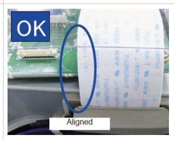
**4.** Check the long ribbon cables back at the main board. They should run parallel to the main board.
