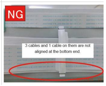
**10.** Align the outer most cable with the long ribbon cables. You can use masking tape to hold them in place.
