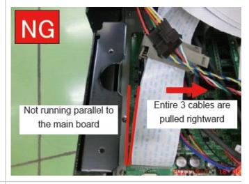
**5.** Check to make sure the long ribbon cables are aligned with each other.
