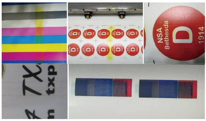
The cause of the issue is a misalignment in the long data cables which send the signal to the print heads. The misalignment causes a digital noise which causes print quality issues. The misalignment has also been attributed to print and cut accuracy issues as well.
