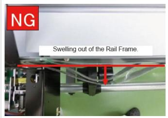
**12.** Correct cable positioning to be as shown.
