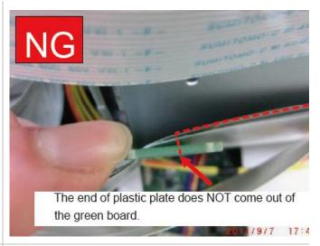
**14.** If the insulation cable does not pass through the green board make the correction so it appears as it does in the image by following the next steps. If it is ok, the process is complete.
