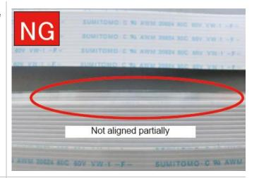
**8.** Align ribbon cables along the length of the rail frame. Use masking tape to align the cables if needed.
