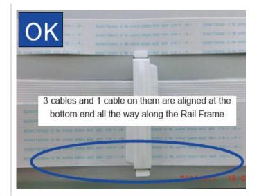
**11.** Check to make sure all cables are not swelling out from the rail frame as shown.
