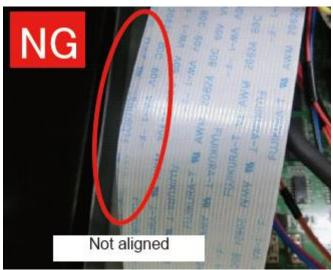
**6.** Align long ribbon cables with each other and make them parallel with the main board.
