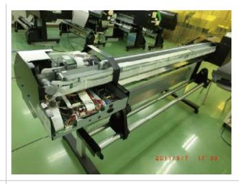
**2.** Check the alignment of the long ribbon cables at the print carriage board.
