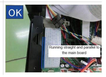
**7.** On the back side of the printer check the path of the long ribbon cables and make sure they are aligned. The tolerance is within one signal line.
