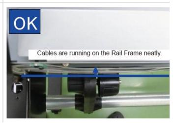
**13.** On the capping station side of the printer there is a plastic plate. Make sure the clear insulation cable passes through the green board.
